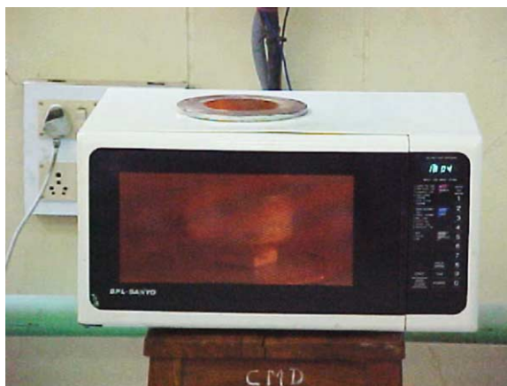
Fig. 1. Modified domestic microwave oven used for the powder synthesis.
