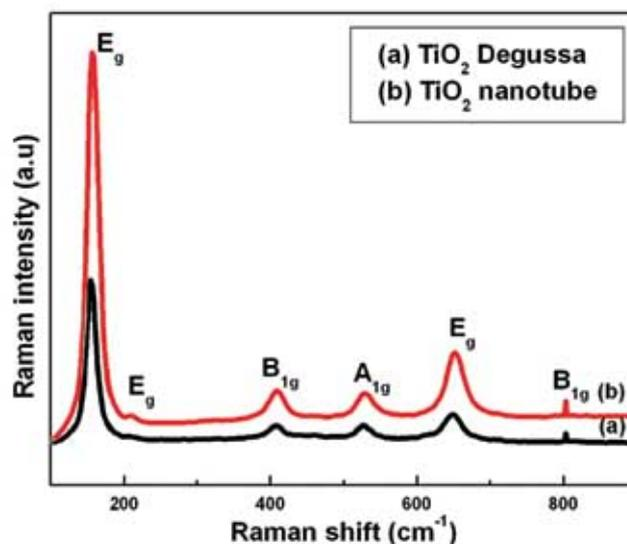
**Figure 4.** Raman spectrum of (a) Degussa TiO<sub>2</sub> and (b) fabricated anatase-TiO<sub>2</sub> nanotube (The vibration mode symmetries of the anatase are indicated).
