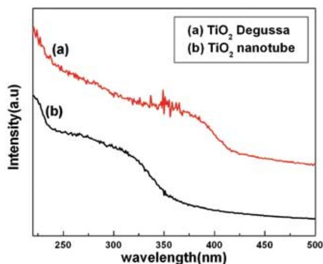
**Figure 2.** UV-*vis* absorption spectrum of (a) Degussa TiO<sub>2</sub> and (b) anatase TiO<sub>2</sub> nanotube.
