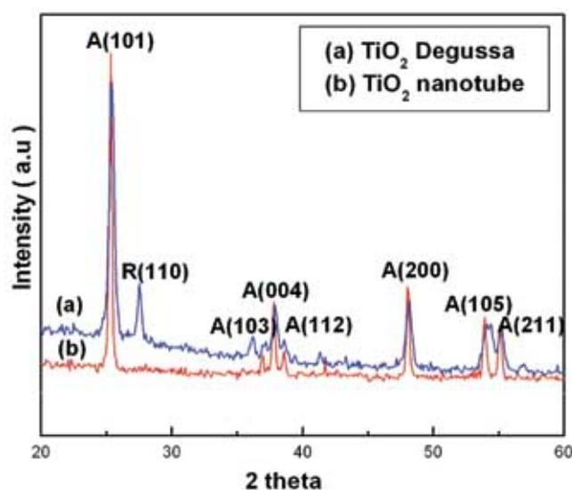
**Figure 3.** X-ray diffraction patterns of (a) Degussa TiO<sub>2</sub> as a reference and (b) TiO<sub>2</sub> nanotubes obtained by sol-gel method calcined at 650 °C for 2 h anatase phase.
