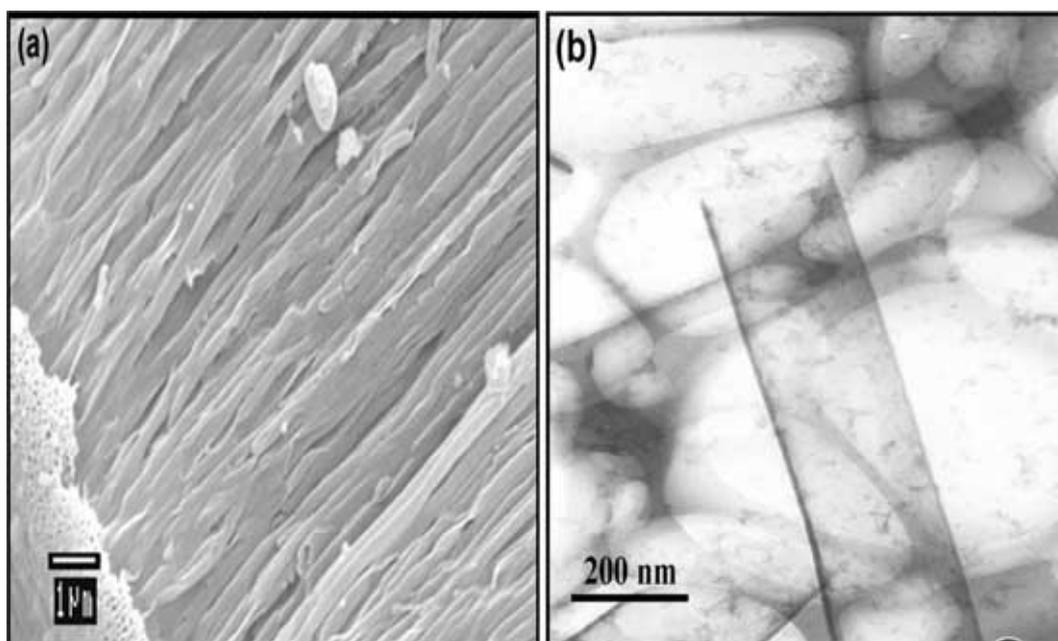
**Figure 1.** SEM image (a) and TEM image (b) of  $\text{TiO}_2$  nanotubes obtained by sol-gel method calcined at  $650^\circ\text{C}$  for 2 h.
