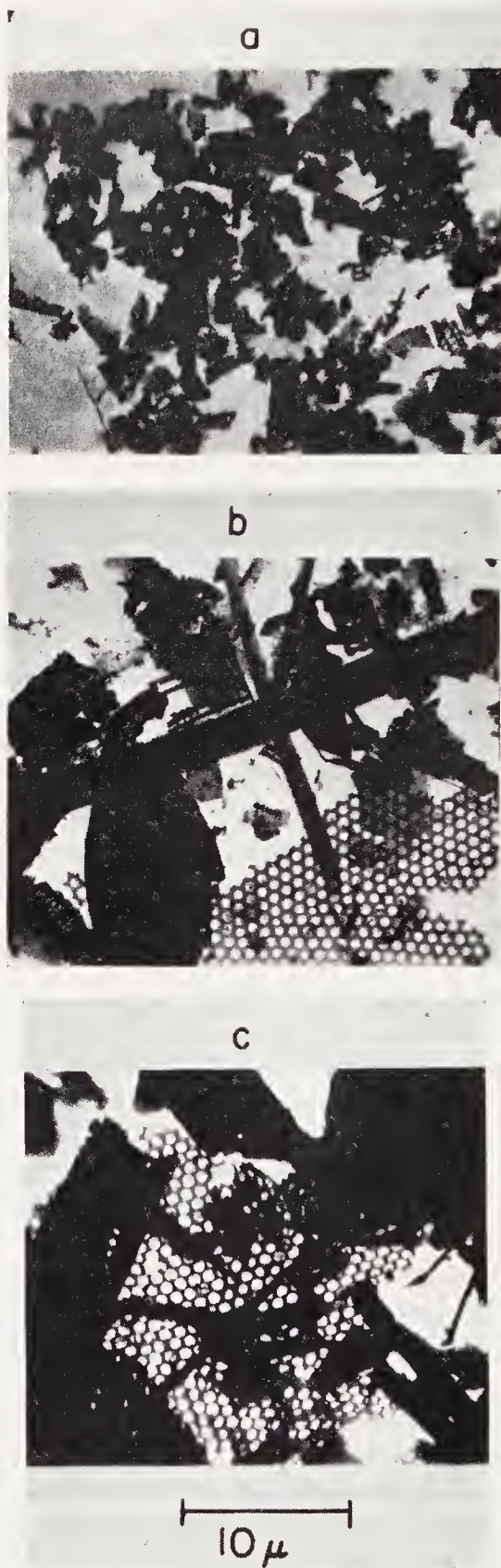
Figure 9. Electron micrographs of kieselguhrs at a magnification of 2,000. Natural kieselguhrs— a . "Snow Floss" b . "Filter Cel" Flux-calcined kieselguhr— c . "Hyflo-Super-Cel"
