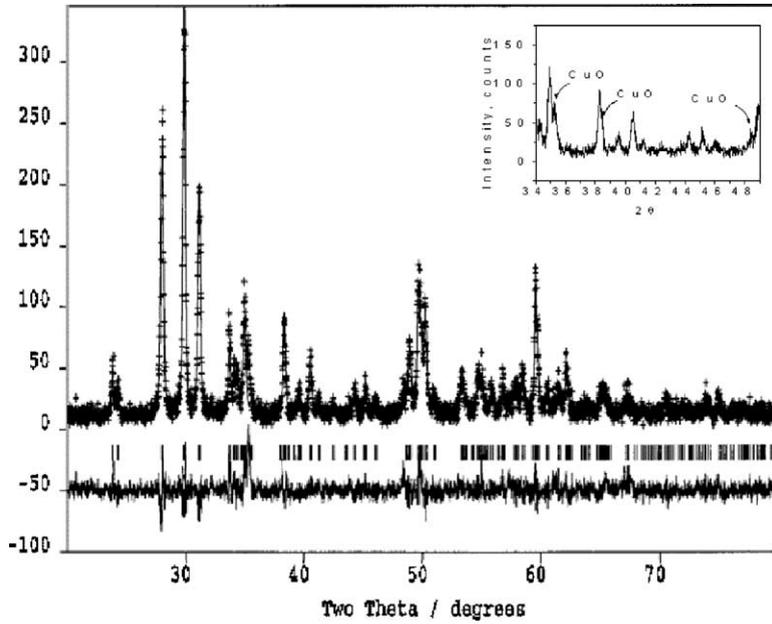
Fig. 7. Rietveld refinement of  $\text{CuZr}_{20}$  sample scanned at 1173 K.
