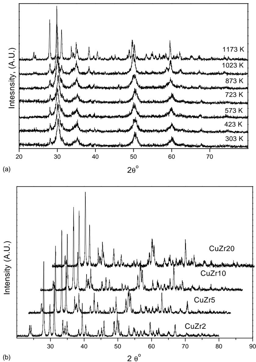
Fig. 6. (a) Multiple plots of the powder XRD patterns of the  $\text{CuZr}_{20}$  sample scanned at various temperatures. (b) Multiple plots of the  $\text{CuZr}_2$ ,  $\text{CuZr}_5$ ,  $\text{CuZr}_{10}$ , and  $\text{CuZr}_{20}$  samples scanned at 1173 K.
