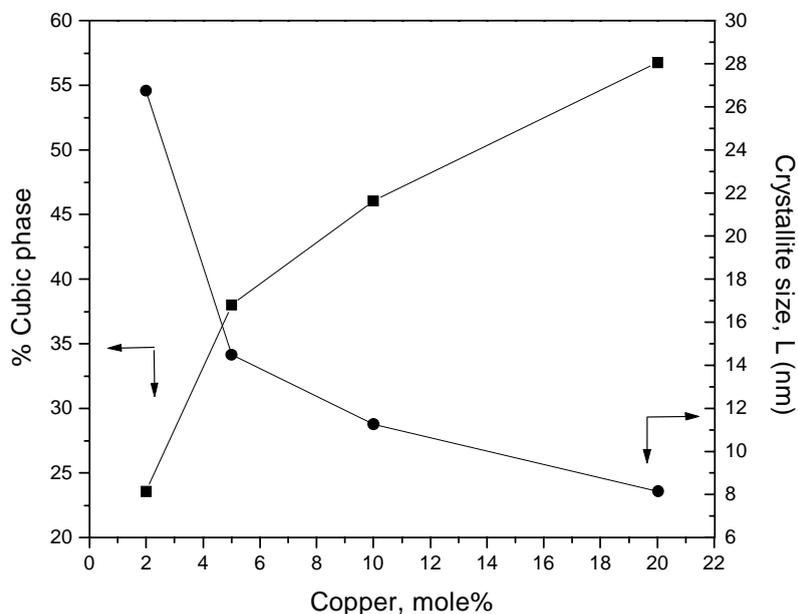
Fig. 5. Change in the crystallite size and the relative percentage of the cubic phase with varying copper content. (■) Percent of cubic phase; (●) crystallite size.
