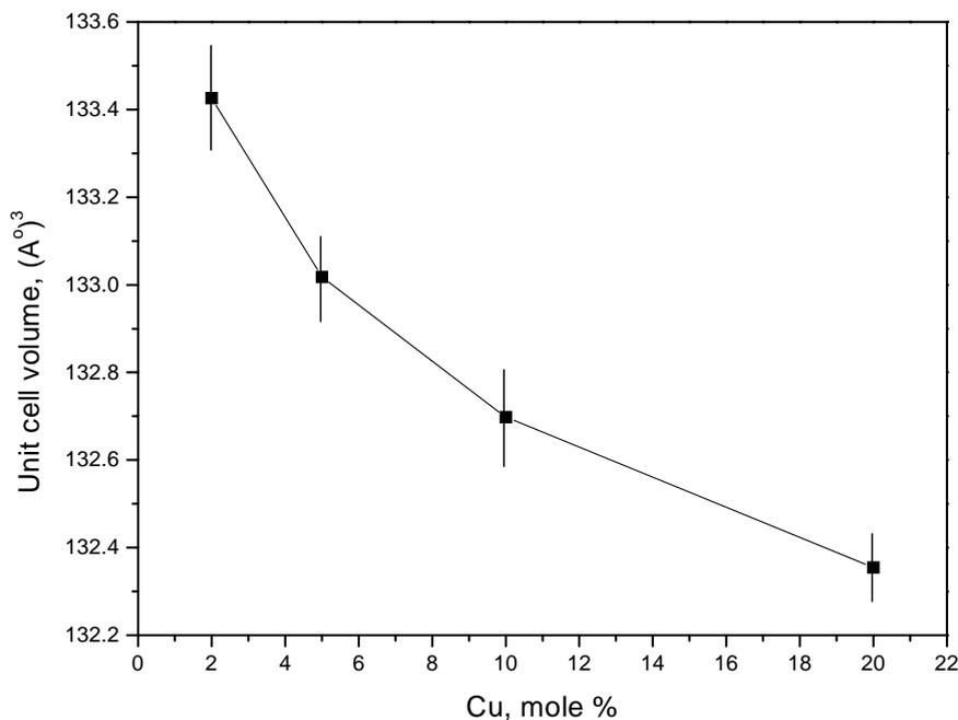
Fig. 4. Change in the unit cell volume of the cubic phase as a function of the copper concentration.
