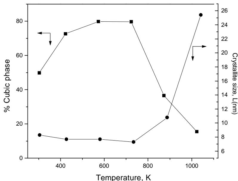
Fig. 9. Change in the percentage of the cubic phase and the crystallite size as a function of temperature. (■) Percent of cubic phase; (●) crystallite size.
