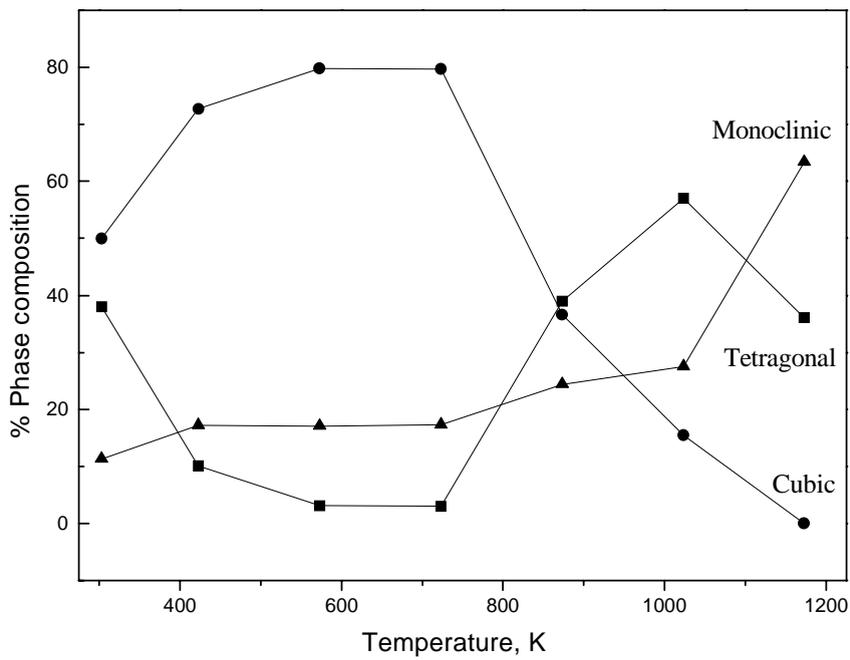
Fig. 8. Changes in the relative phase compositions of the samples with the increasing temperature. (■) Tetragonal; (●) cubic; (▲) monoclinic.
