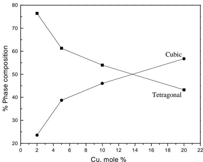
Fig. 3. Change in the relative concentration of the tetragonal and cubic phases as a function of copper concentration in zirconia. (■) Tetragonal; (●) cubic.
