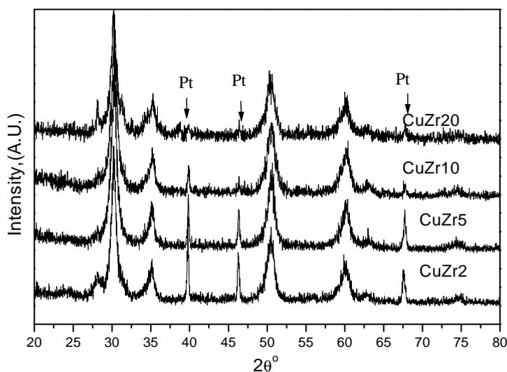
Fig. 1. Multiple plots of the powder XRD patterns of the zirconia samples containing 2, 5, 10, and 20 mol% copper, respectively. Reflections from Pt are indicated.
