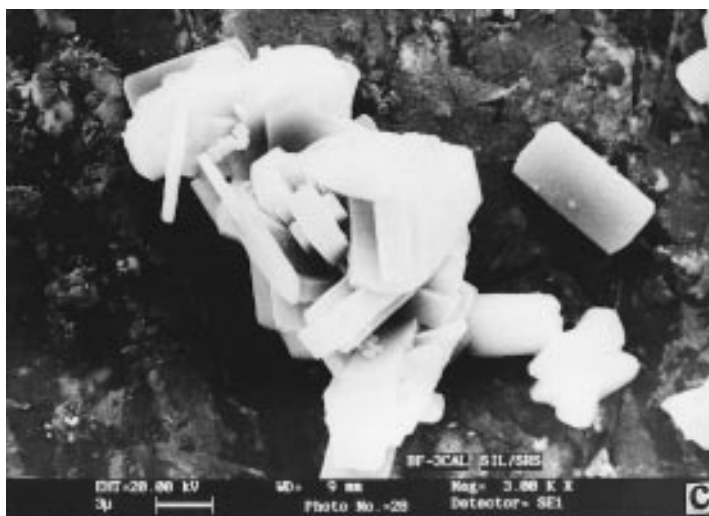
Figure 2. Scanning electron micrographs of Zr-Sil-1 sample A (a), sample D (b), sample F (c) and Sil-1 (d). (Continued on next page.)
