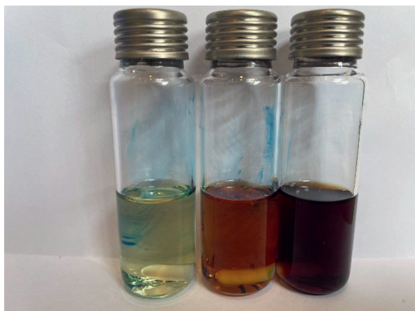
Figure 2.9: left to right: acetic acid – triethylamine (1.5:1 molar ratio), acetic acid – triethylamine (3:1 molar ratio) and propionic acid – trioctylamine (1.5:1 molar ratio), after 1 week.
