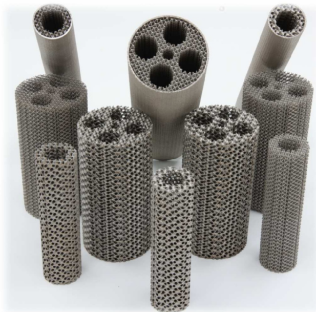
Figure 1-9: POCS Support for Ambher EU Project proof of concept, 3D-Printed by ENGIE Laborelec using Selective Laser Melting with Kelvin Cell design [83] (featuring gyroid and BCC lattices and holes for the membranes & thermocouple integration)
