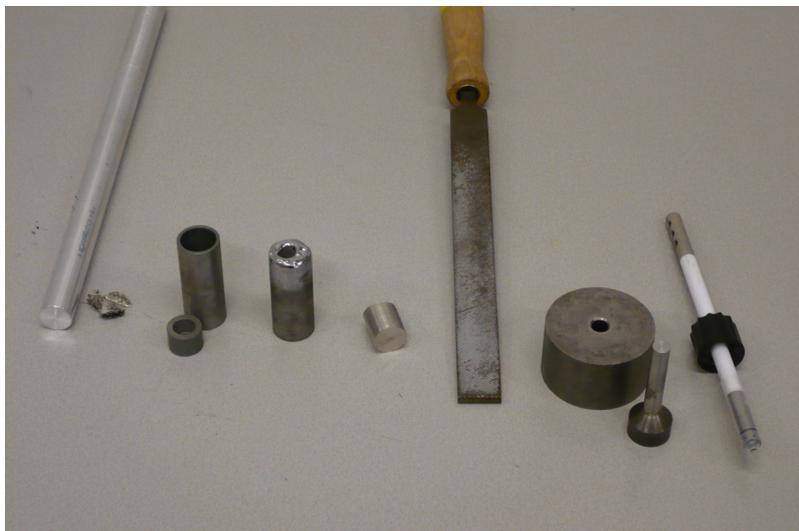
Fig. 9: From left to right: Mg rod and Sc pieces, Mo crucible with lid, sealed Mo crucible, ingot after removal of Mo crucible, file to shave off small metal pieces to make working electrodes, mold to press active material and metal powder into a pellet, electrode holder with pellet fixed at the end by a shrink sleeve.
