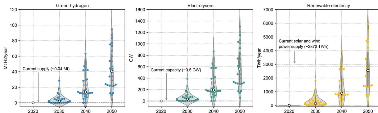
**Fig. 3.** Resource and infrastructure requirements for meeting the expected global demand for green hydrogen-based steel derived from 28 scenarios. White symbols represent the median of the data, while the thick grey bars represent the interquartile range. The thin grey area shows the distribution of the data using kernel density estimation. (For interpretation of the references to colour in this figure legend, the reader is referred to the Web version of this article.)
