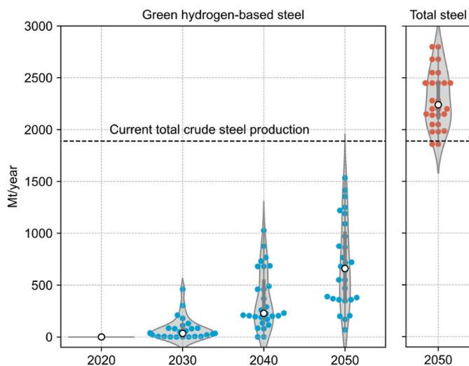
**Fig. 2.** Expected global demand for green hydrogen-based steel derived from 28 scenarios. White symbols represent the median of the data, while the thick grey bars represent the interquartile range. The thin grey area shows the distribution of the data using kernel density estimation. (For interpretation of the references to colour in this figure legend, the reader is referred to the Web version of this article.)
