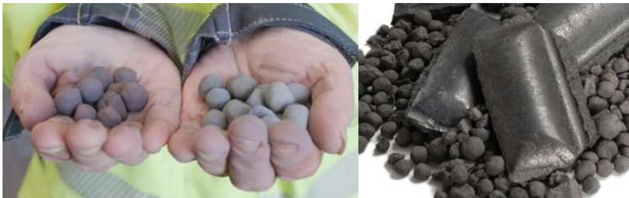
Figure 9: Left: Ore pellets on the left, and DRI pellets on the right (note the color change, from reddish to greyish). Right: Hot briquetted iron. Source: (HYBRIT, 2024a)
