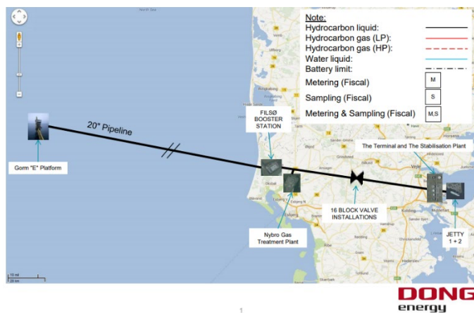
Figure 0-16: Oil transportation system [17]
