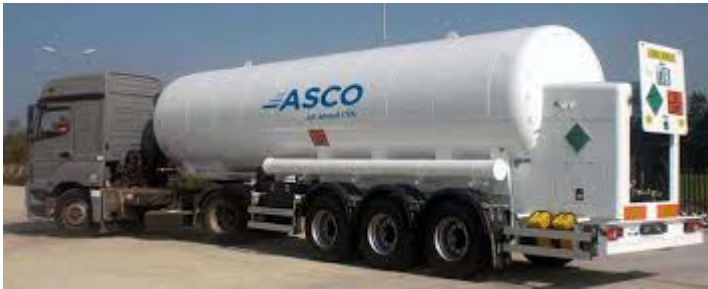
Figure 50. CO 2 semi-trailer from ASCO. Source; www.ascoCO2.com
