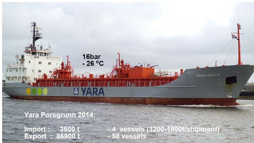
Figure 49. M/T Yara Gas III liquid CO 2 carrier. [7]
