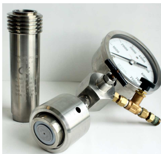
Figure 1. Autoclave for ammonothermal and hydrothermal reactions.
