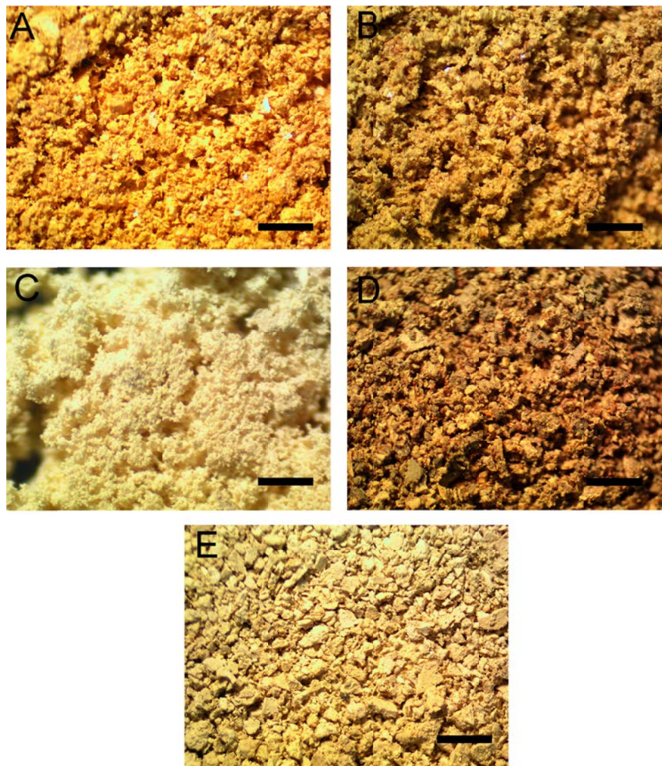
Figure 3.14 – Optical microscope images of C 3 N 4 products from 500 °C tube decomposition of (A) TCM-NaCl, (B) TCM-KBr, (C) TCM-KI, (D) TCM-KSCN, and (E) TCM-NH 4 SCN. Scale bar represents 2 mm.
