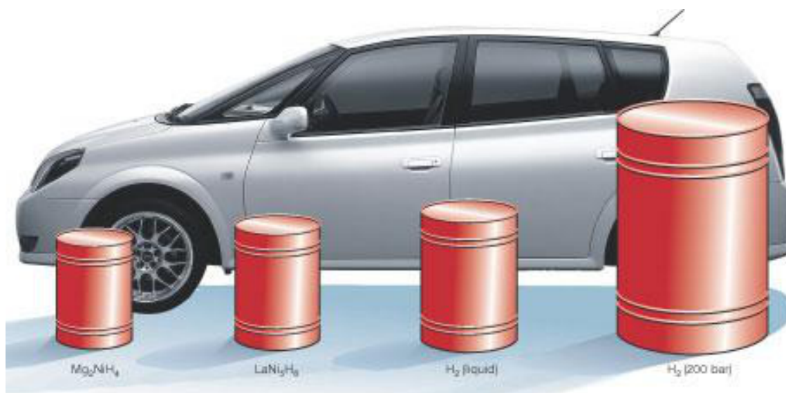
Figure 1.1 Volumetric comparison of several current methods of storing 5 kg of hydrogen, an amount suitable for use in a personal vehicle. 13
