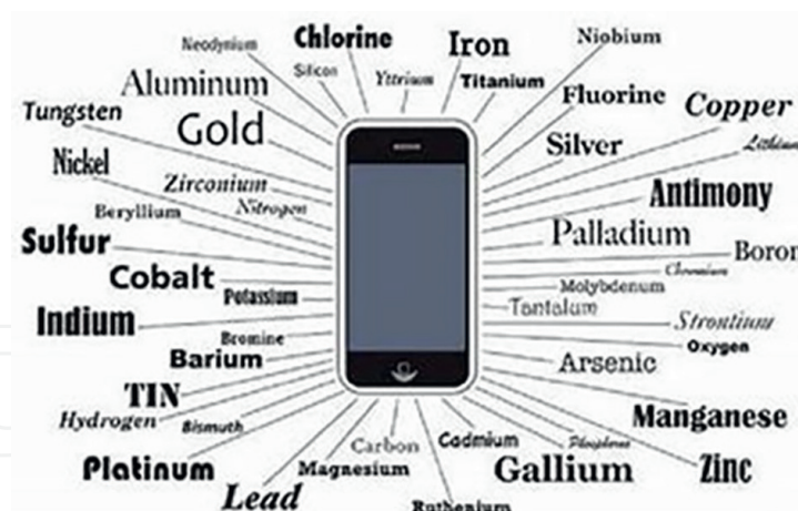
Figure 1. Estimated materials in one iPhone require 46 different elements reported according to Stanford Advanced Materials (SAM) Corporation [2].
