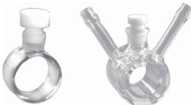
Figure 5.56 Water-cooled cylindrical 20-ml quartz cuvettes with (a) and without a cooling jacket (b).
