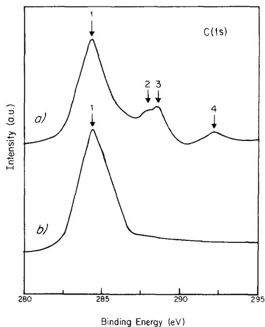
Fig. 3. XP spectra of FeTi alloy under different experimental conditions: (a) air exposed and (b) oxygen exposed. The peak numbers represent the same assignments as described in Fig. 1.
