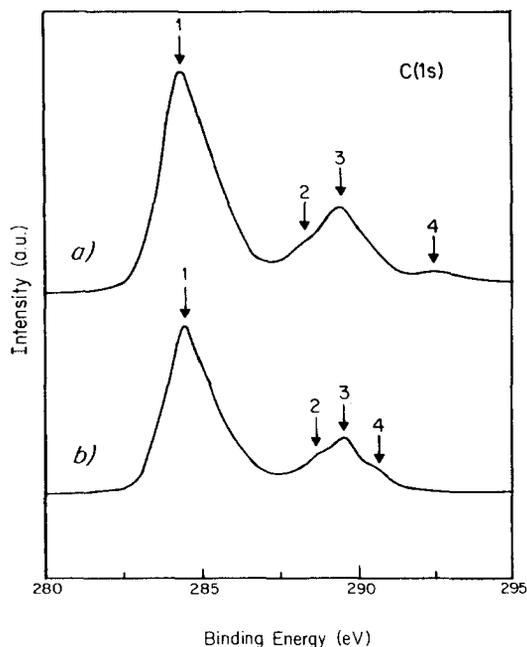
Fig. 2. XP spectra of air exposed samples: (a) Mg<sub>2</sub>Ni and (b) Mg<sub>2</sub>Cu. The peak numbers carries the same assignments as described in Fig. 1.
