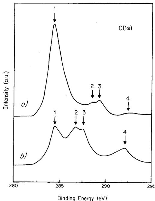
Fig. 1. XP spectra of air exposed samples of: (a)  $\text{LaNi}_5$  and (b)  $\text{CaNi}_5$ . The numbers represent the nature of different signals: 1-reference carbon; 2-, 3- and 4-carbon dioxide adsorbed on different sites (see text).
