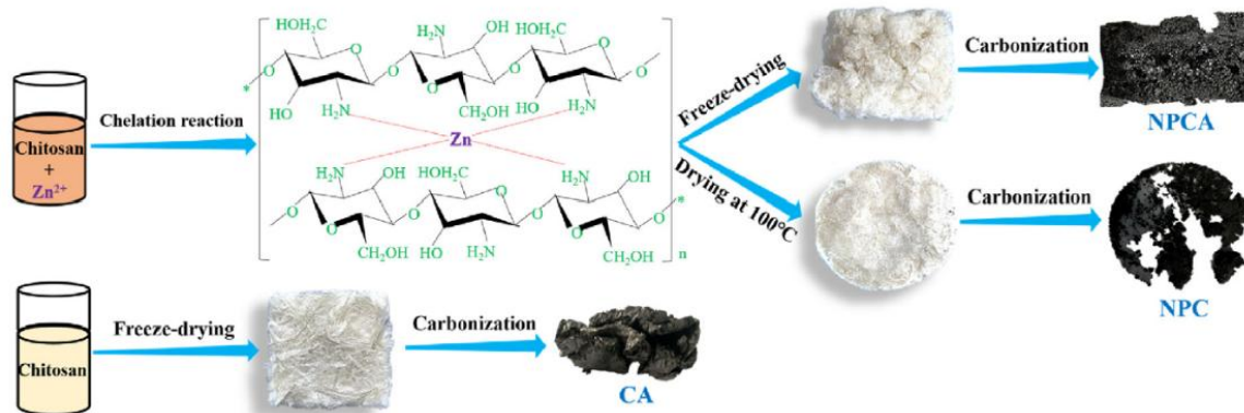
Figure 3 The schematic synthesis routes of NPCA [30]
