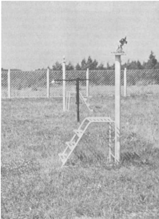
Fig. VII.1. Sensor for reflected solar radiation (left) registering data to be subtracted from measurements of incoming solar radiation to give the amount of solar energy absorbed by the grass, here on the observation field of the Glavnaia Geofizicheskaia Observatoriia at Voeikovo near Leningrad. Beam radiation is measured by pyrliometer on post at right.
