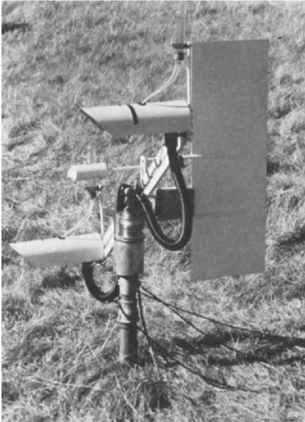
Fig. XXIII.3. Bowen-ratio meter above native Themeda grassland at Krawarree in the Southern Tablelands of New South Wales. Shielded wet- and dry-bulb thermometers at two levels are periodically interchanged to avoid systematic error in determining vertical differences in temperature and specific humidity for the Bowen allocation of energy to latent- and sensible-heat fluxes.
