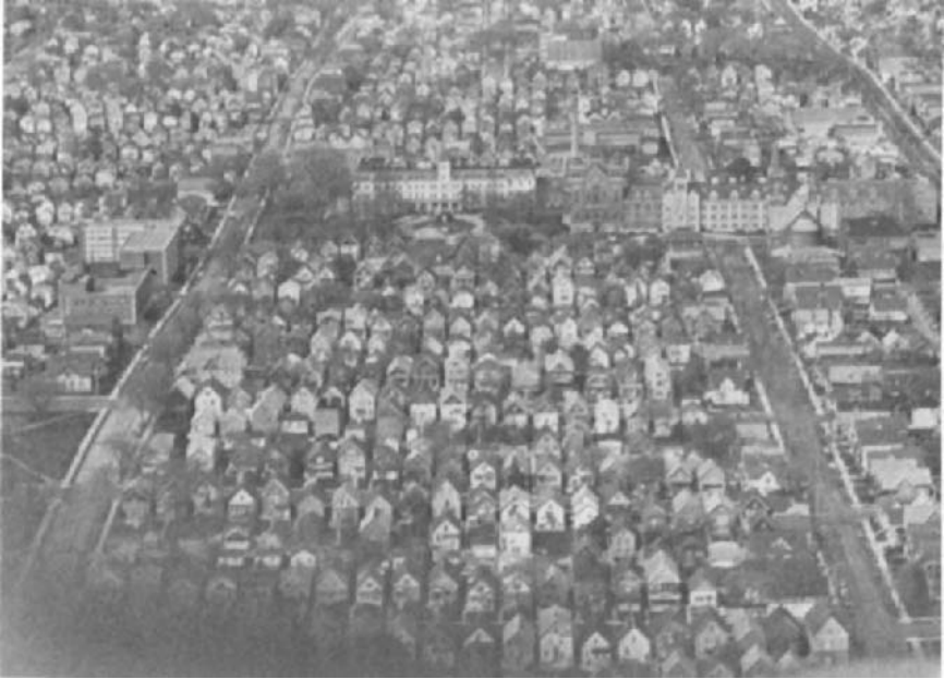
Fig. XXII.3. East-facing ends of Milwaukee houses lit by the morning sun at 1030, 23 April 1976, as seen from 150 m. This orientation is efficient from a standpoint of solar geometry.
