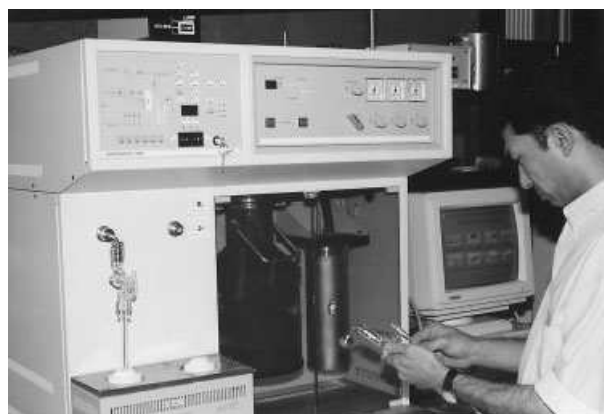
Fig. 5-44 Sorptometer (catalysis laboratory, FH Mannheim, Germany)
