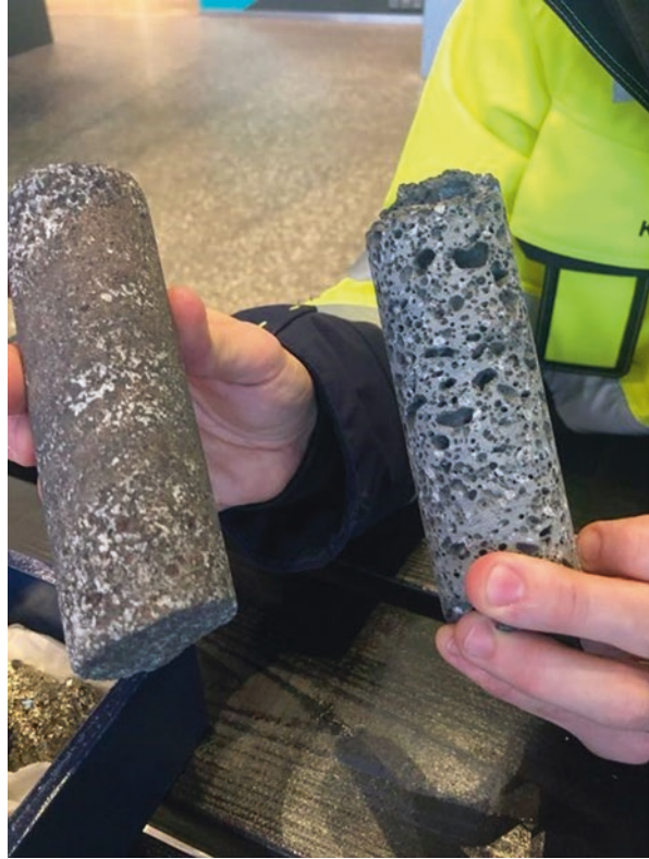
Fig. 9.4 Iceland basalt core on the left shows vesicles filled with precipitated white carbonate minerals; core on the right shows porous vesicular basalt before carbon dioxide was introduced to the system Image source: Carbfix, U.S. Department of Energy (public domain)
