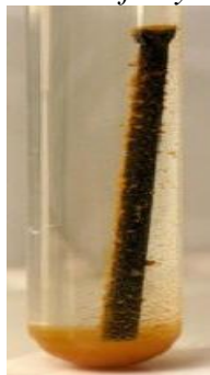
1 Red-brown flaky rust
