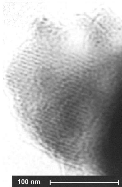
Figure 2. TEM image of calcined (Cr)HMA catalyst.
