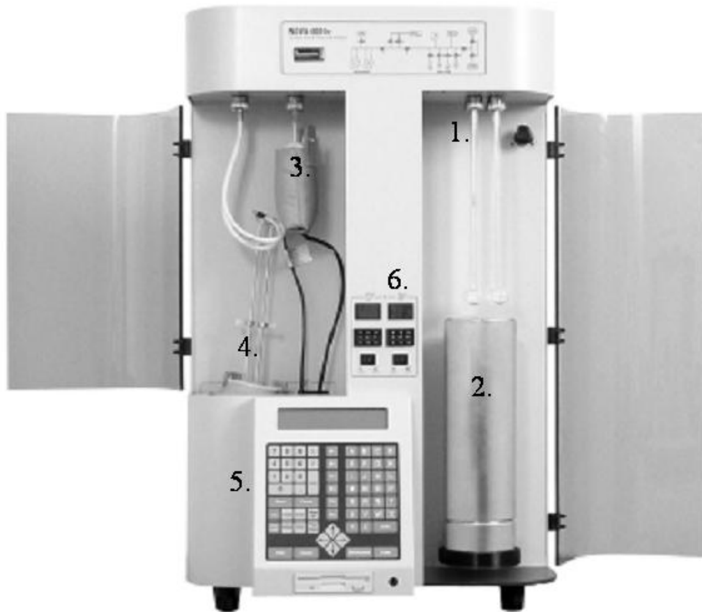
Figure 3.5. Nitrogen sorption analyzer and its main constituent parts: 1) sample cells, 2) an open-ended Dewar with liquid nitrogen, 3) a sample cell placed in the heater in process of vacuum degassing, 4) a sample cell placed in the heater in process of nitrogen flow degassing, 5) a keyboard control unit, 6) a temperature controller.
