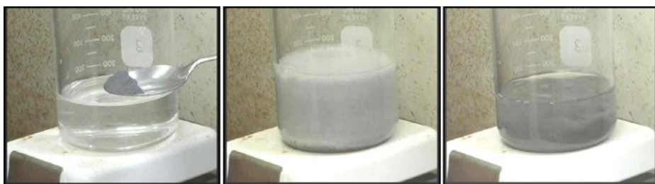
Figure 2.5: Activation of powdered Ni–Al alloy added to NaOH solution. Photo by Edward Laughlin.
