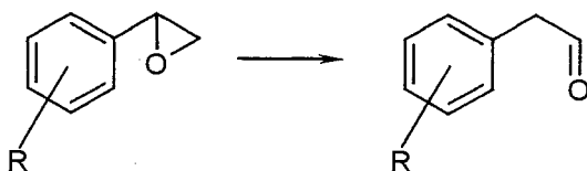
Figure 2. Rearrangement of styrene epoxides (R = alkyl, aryl, haloalkyl, alkoxy, alkylthio).
