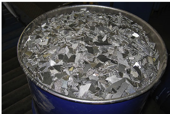
FIGURE 28.1 Cobalt metal, produced electrolytically in the Democratic Republic of Congo. Photograph courtesy of Katanga Mines Limited.
