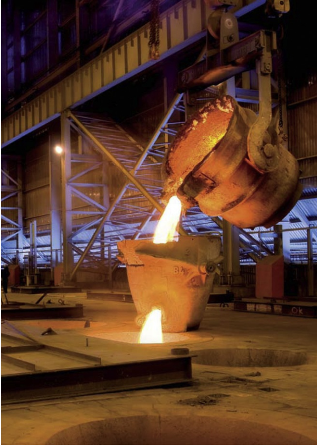
FIGURE 21.4 Casting of low-iron, sulfur-deficient matte into floor-level molds in preparation for slow cooling. Slow cooling causes the matte to separate into \sim 100\ \mu\text{m} \text{Cu}_2\text{S} , \text{Ni}_3\text{S}_2 and alloy grains, which are separated by comminution then magnetic separation and froth flotation. The alloy grains contain most of the silver, gold and platinum-group elements in the matte. The newly-filled molds will be covered with the lid (left). Photograph courtesy of Anglo American Platinum.
