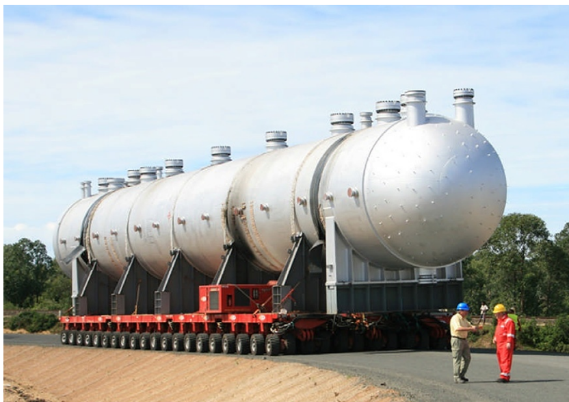
FIGURE 11.4 High-temperature sulfuric acid leaching autoclave moving toward laterite leach plant in Ambatovy, Madagascar. Note that almost all access into the autoclave is through the top.
