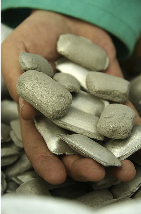
FIGURE 1.7 Nickel briquettes produced from powder obtained from the hydrogen reduction of nickel in solution (see Chapter 27). An important alternative process is electrowinning, which is discussed in Chapter 26. Photograph by M. Fox, courtesy of Impala Platinum.
