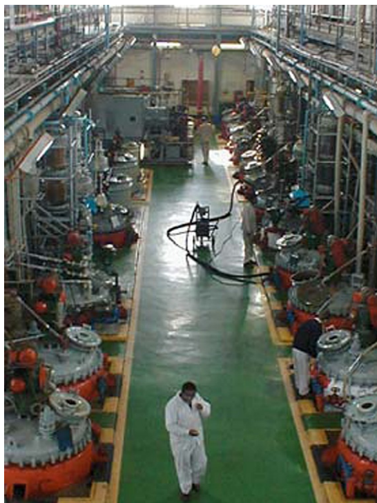
FIGURE 37.6 A view of the production facilities at Lonmin's Western Platinum Refinery. The glass-lined reactors are arranged on either side of the production hall of the primary separations plant. Generally, the filtration steps are carried out on the level below this. However, a variable chamber filter can be seen at the back of this hall. Note that the requirements for personal protection equipment have become more stringent since this photograph was taken. Photograph courtesy of Lonmin plc.
