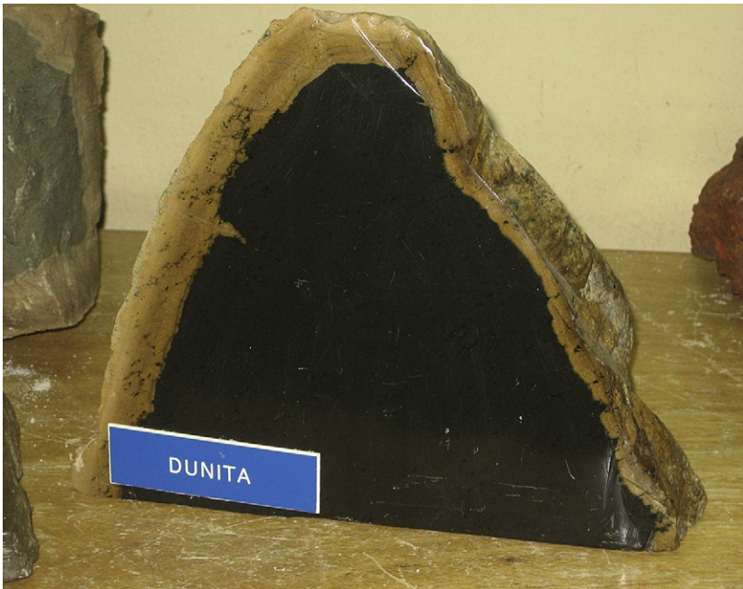
FIGURE 3.4 Partially laterized dunite rock, consisting mainly of olivine [(\text{Mg},\text{Ni})_2\text{SiO}_4] . The outer skin is typically garnierite [(\text{Mg},\text{Ni})_3\text{Si}_4\text{O}_5(\text{OH})_4] . Garnierite can be removed from the dunite by gentle crushing and grinding. Source: Photograph by W.G. Davenport.
