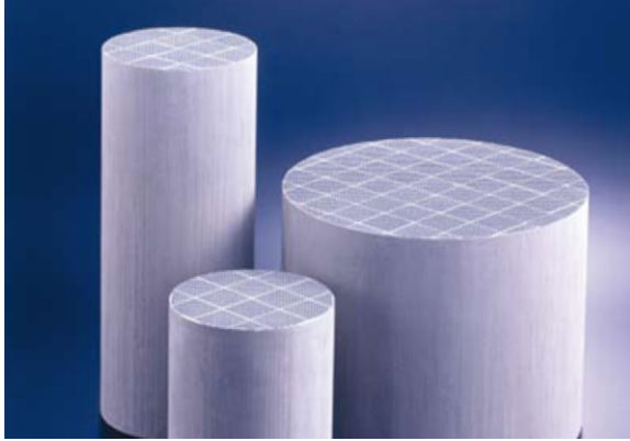
FIGURE 38.1 Ceramic car/truck catalyst substrate blocks. They are mostly made of cordierite, Mg_2Al_4Si_5O_{18} , which has a low coefficient of thermal expansion (Kendall, 2004). Their pores are coated with nanoparticles of platinum, palladium and rhodium. The platinum-, palladium- and rhodium-coated substrates are recycled for the recovery of these metals after their host vehicles have been scrapped (Figures 1.6 and 38.2).
