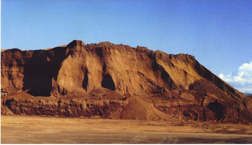
FIGURE 3.2 Upgraded saprolite ore from New Caledonian, containing about 3% Ni. This material has been upgraded from ore containing 1.8% Ni. It is destined to be smelted and refined to produce ferronickel, containing 30% Ni and 70% Fe, which is used mainly for making stainless steel. Source: Photograph courtesy of Société Le Nickel-SLN/Eramet.
