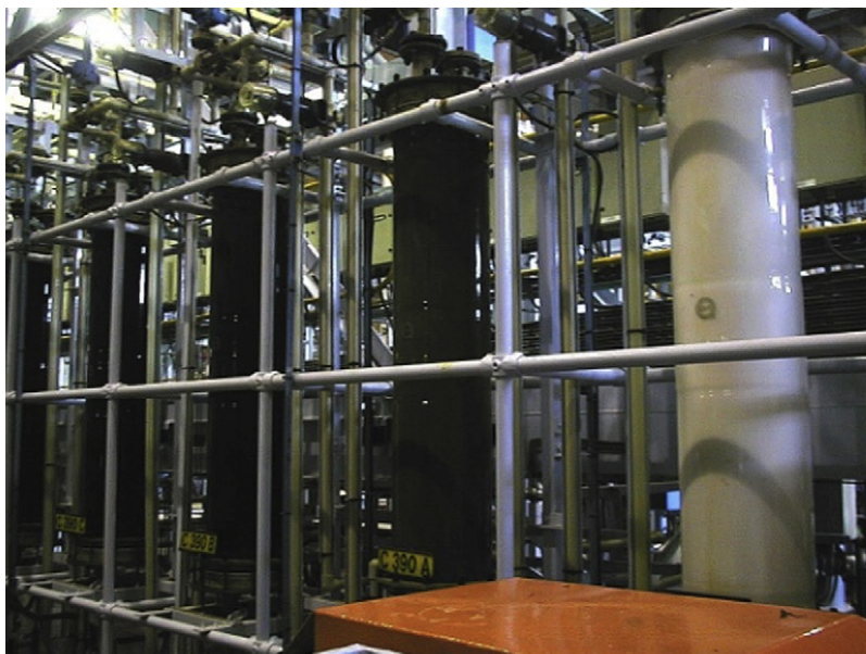
FIGURE 37.3 Ion-exchange columns for the separation of gold from solution. The columns are arranged in a lead–middle–trail configuration. Three columns are used in series – the first is the lead and the last is the trail column. Once the lead column is fully loaded, the middle column becomes the new lead, the trail column becomes the new middle, and the lead is eluted and becomes the new trail column. Photograph courtesy of Impala Platinum.
