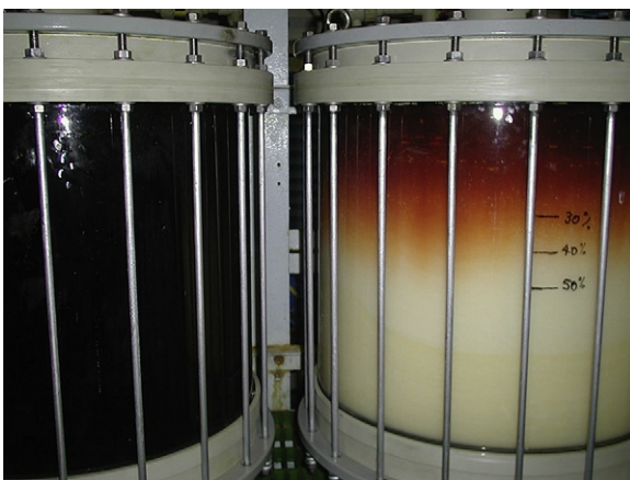
FIGURE 37.14 A close-up of the ion-exchange columns, showing an extraction front in the column on the right-hand side. This front indicates palladium that has loaded onto the SuperLig 2. The column on left-hand side is fully loaded. Photograph courtesy of Impala Platinum.
