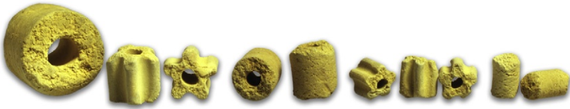
FIGURE 20.2 Photograph of catalyst pieces used in the oxidation of sulfur dioxide. The outside diameter of the largest piece is 20 mm. The pieces are used in ~1 m thick, ~10-m-diameter beds in stainless-steel towers. Rings, star rings and pellets are shown. The star rings maximize catalyst area and minimize resistance to gas flow. At temperatures of 420°C–620°C, a molten layer of vanadium–alkali metal sulfate/pyrosulfate covers the porous solid silica substrates. Photograph courtesy of Haldor Topsoe A/S.
