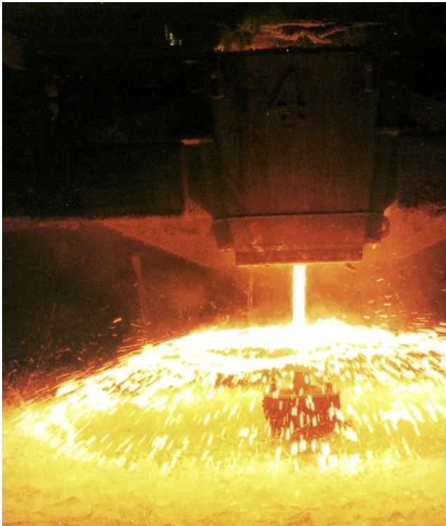
FIGURE 7.2 Production of ferronickel 'beans' by controlled pouring of molten ferronickel into a spinning refractory cup and on into water. The product is flat, \sim 0.03 m diameter \times 0.005 m thick 'beans' suitable for controlled addition into alloy-making ladles or furnaces. Source: Photograph courtesy of Pacific Metals Co., Ltd., Hachinohe, Japan.
