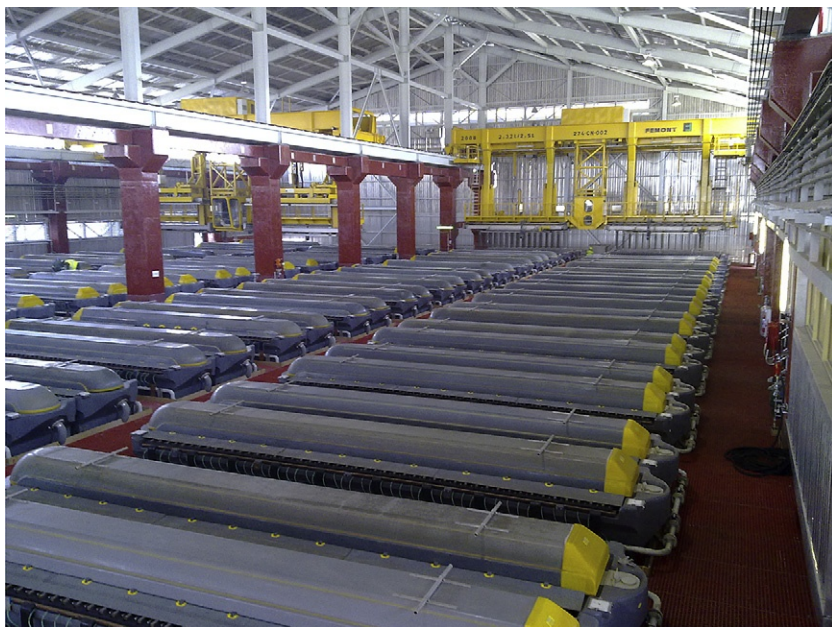
FIGURE 26.5 The nickel tankhouse at Anglo American Platinum, showing the mist abatement hoods and the crane for automatic harvesting of the nickel cathodes. Source: Photograph by J. J. Taute, courtesy of Anglo American Platinum
