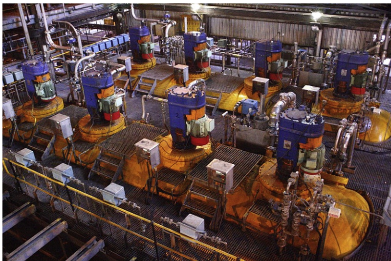
FIGURE 36.7 Two of the autoclaves used for leaching at Impala Platinum. Photograph by M. Fox, used with permission of Impala Platinum.
