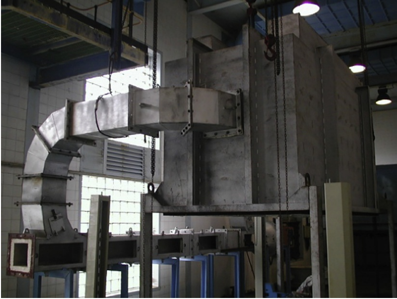
FIGURE 37.4 An ignition furnace at Impala Platinum. Note the off-take ducting on the left-hand side of the furnace for the extraction of gases.
