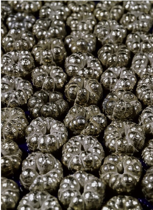
FIGURE 26.3 Nickel crowns produced by masking titanium mother blank cathodes with polymer then electrowinning. Photograph courtesy of Xstrata Nikkelverk.
