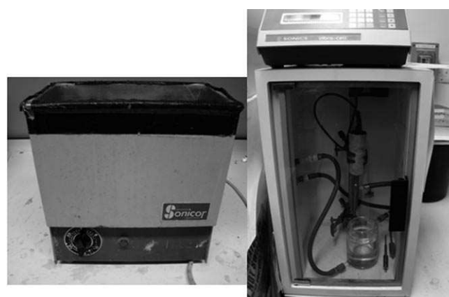
Figure 10. Traditional ultrasonic bath (left) and ultrasonic probe (right) employed for the preparation of supported metal nanoparticles.
