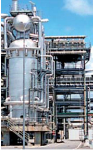
Water cooled (steam rising) multitubular reactor for methanol synthesis
