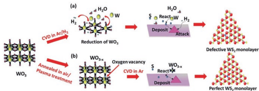
Fig. 8.3 Effects of precursor pre-treatment on the vapor deposition of WS 2 monolayers. (Reprinted from Ref. [32]. Copyright 2019, The Royal Society of Chemistry . Available under Creative Commons Attribution-Non Commercial 3.0 Unported License, https://creativecommons.org/licenses/by-nc/3.0/ )
