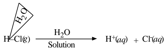
Figure 7.5 HCl dissolving in water. Water breaks apart a hydrogen chloride molecule to form a hydrogen ion, H^+ , and a chloride ion, Cl^- .
