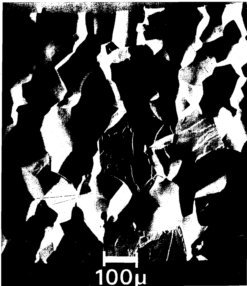
Figure 7.6 SEM micrograph of intergranular and intra-crystalline cleavage in \alpha -iron (micrograph edge 0.75 \text{ mm} )
