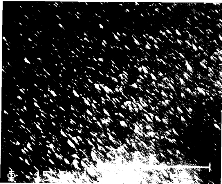
Figure 6.7 Secondary electron image of the Al-Cu film before heat treatment, after etching the sample by argon ion bombardment to a depth of approximately 11 000 Å. Note that the small cone structures point in the direction of the incident ion beam.
