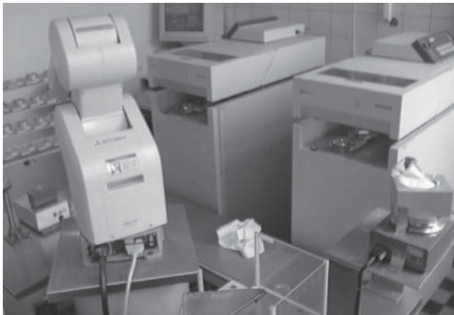
Figure 18.6 Fusion automat with two inductive heated fusion instruments.
