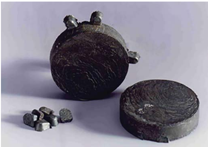
Figure 3.5 Specimen generated by sampling from a melt.
