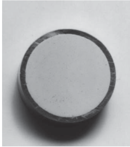
Figure 18.4 Pressed pellet from powder material in a ring of steel as a result of automated preparation process.
