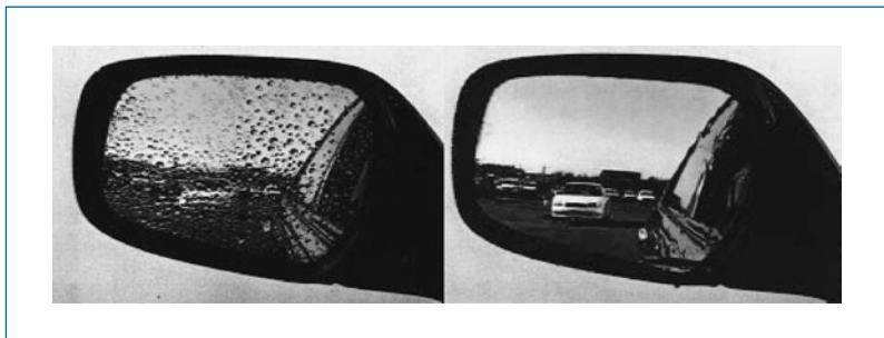
Fig.19. Anti-fogging effect of automobile side-view mirror: conventional mirror (left) and TiO 2 -coated mirror (right).
