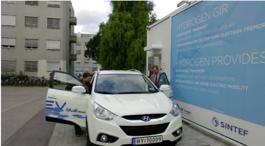
Fig. 2.6 The Hyundai ix35 Fuel cell Electric Vehicle. This car is fuelled with 700 bar hydrogen gas. It is photographed at the SINTERF Headquarters in Oslo. Source Bartek Glowacki)
