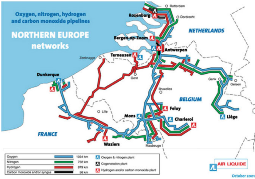
Fig. 6.3 Northern Europe hydrogen pipelines. Source Wiley with permission, image from [5] © Air Liquide
