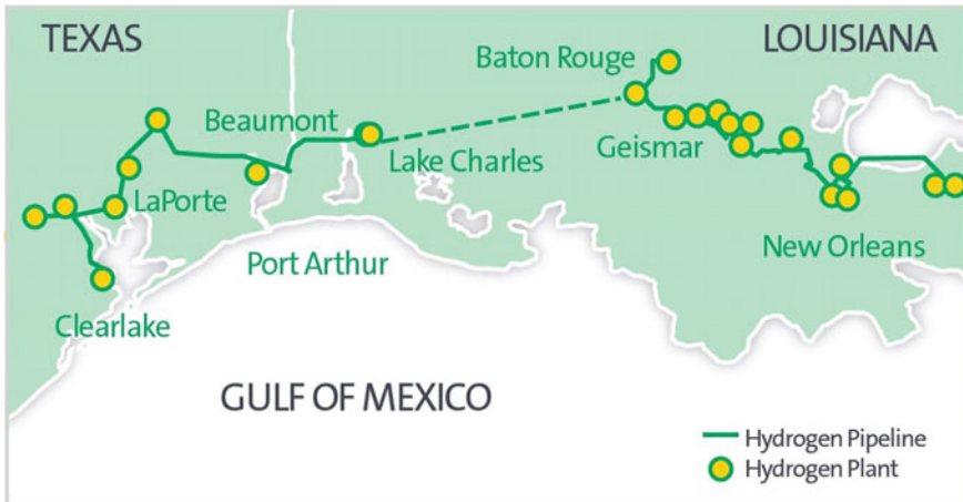
Fig. 6.5 Air Products' hydrogen pipeline runs for more than 180 miles along the US Gulf Coast. Source From [11]
