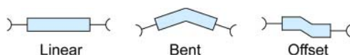
Figure 3.6 Ditopic linkers of linear, bent, and offset geometry. In addition to the position and angle of the binding groups with respect to each other, the dihedral angle between them has a profound influence on the structure of the product of their reticulation with metal ions (not shown).
