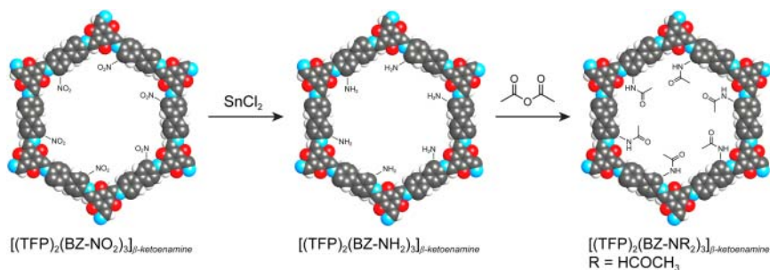
Figure 10.12 Two-step post-synthetic conversion of nitro groups in the mesoporous [(TFP)_2(BZ-(NO_2)_3)]_{\beta\text{-ketoenamine}} : reduction of the preinstalled nitro groups on the linker to amines using SnCl_2 followed by aminolysis of acetic anhydride yield the amide functionalized [(TFP)_2(BZ-((NHCOCH_3)_2)_3)]_{\beta\text{-ketoenamine}} . Owing to the high inherent chemical stability of the frameworks' \beta -ketoenamine linkages and the basic character of the introduced functionalities the resulting materials are utilized for vapor sorption of lactic acid. Color code: H, white; C, gray; N, blue; O, red.
