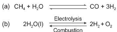
Figure 15.1 Reaction equation for the production of hydrogen gas by (a) steam reforming and (b) electrolysis of water.
