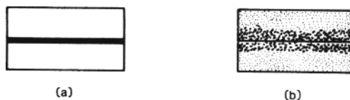
Figure 2.1 A reaction couple used for diffusion experiments. The slabs are carefully polished and oriented slices of MgO. The central dark strip in (a) represents a very thin layer of MgO containing radioactive Mg atoms. After the diffusion experiment the radioactive Mg has moved away from the original plane, as in (b).
