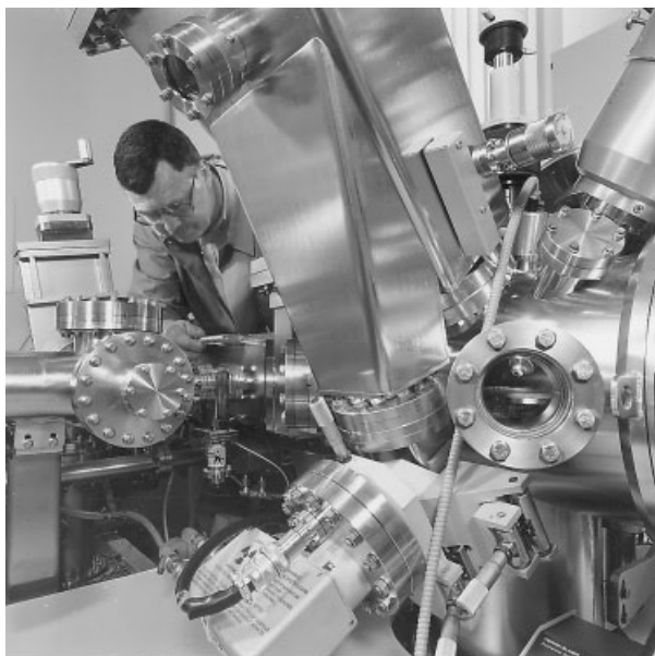
Fig. 5-48 Investigation of a catalyst surface in an ESCA apparatus (BASF, Ludwigshafen, Germany)
