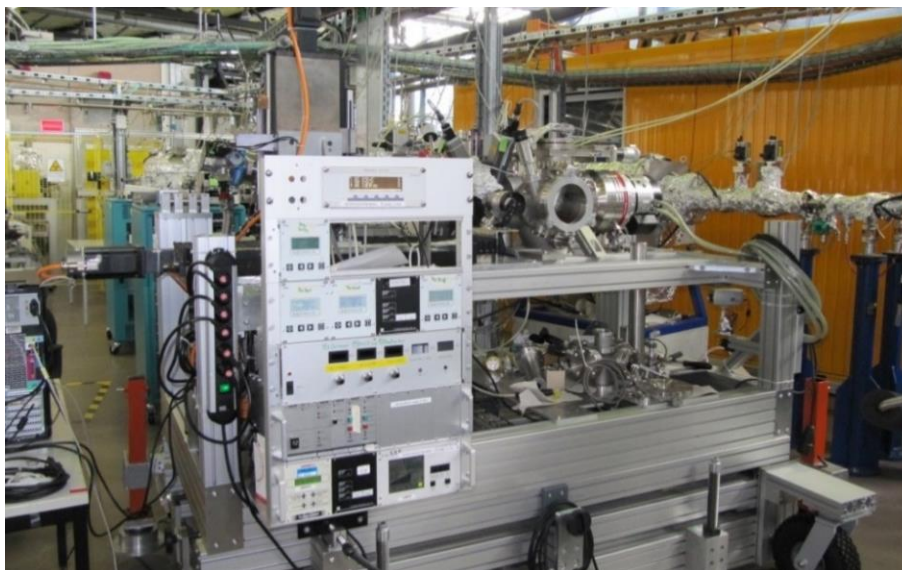
Figure A6 LiXEdrom station in BESSY II synchrotron facility for XAS and RIXS measurements on solids as well as in liquids. Photo was taken by Ronny Golnak, and the permission to use is acknowledged.
