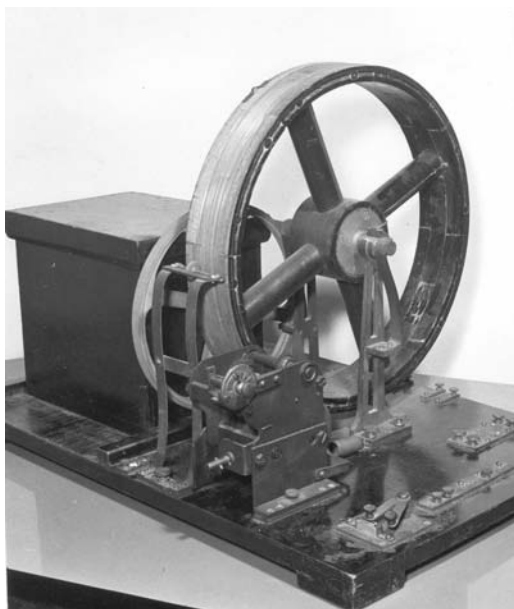
Figure 4.3: The automated polarograph instrument invented by Shikata and Heyrovský.
