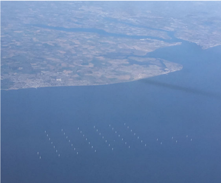
Figure 11.11: Off-shore wind farm Gunfleet Sands with 50 turbines at the English coast of Clacton-on-Sea, Essex. There is 6 \times 7 turbines plus 3 \times 2 turbines of 3.6 MW each, and two new 6 MW turbines. Photo Artur Braun 2017.
