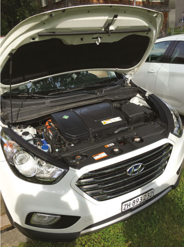
Figure 1.3: Car components under the hood of the Hyundai ix35 Fuel Cell vehicle. The large square-shaped block in the center is the housing of the fuel cell stack.
