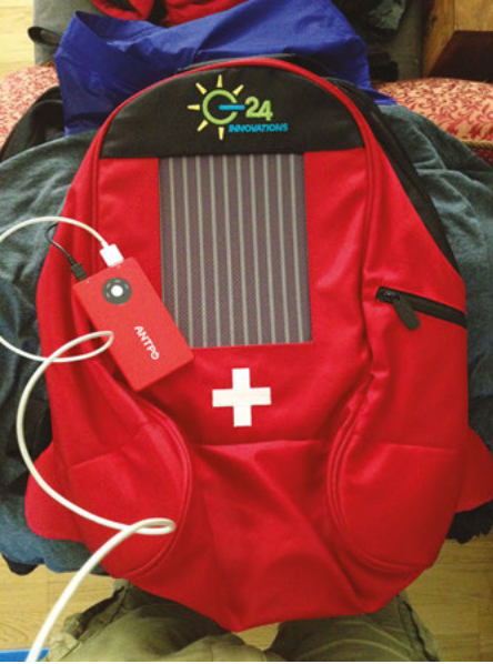
Figure 8.25: This backpack has a DSSC (rectangular lined panel between green-yellow sun and white cross) integrated which charges the small red power bank (lithium ion battery) via the black cable coming from the inside of the backpack. The white USB cable is connected to my iPhone with which I took the photo in April 2015.
