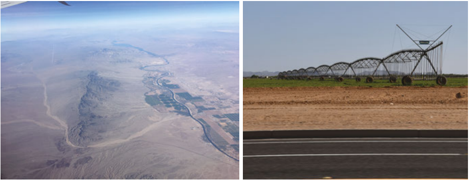
Figure 11.2: (Left) The small city of Needles (5,000 population) in California, at the Colorado River. Dark circles and rectangles are from artificially watered crops and plant fields. The circles can have a diameter of almost 1 km. (Right) Water irrigation machine from 10 segments allowing for circular watering of a crop field.
