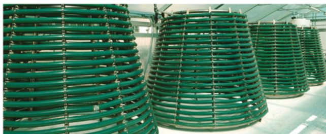
Figure 12.23: Microalgae platform with four photobioreactor units (located at Anhalt University of Applied Sciences, Koethen, Germany).
