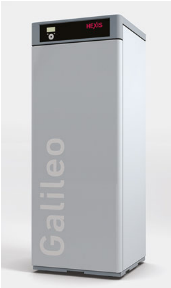
Figure 6.4: “Galileo” SOFC system from the HEXIS AG in Winterthur, Switzerland. The system has the size of a refrigerator. It can be plugged to the natural gas supply in a residential home and produces electricity sufficient to power a home. Around two-thirds of the consumed energy is heat which is used to heat the home and supply warm water. Around one-third of the energy is converted to electric power of 1 kW.
