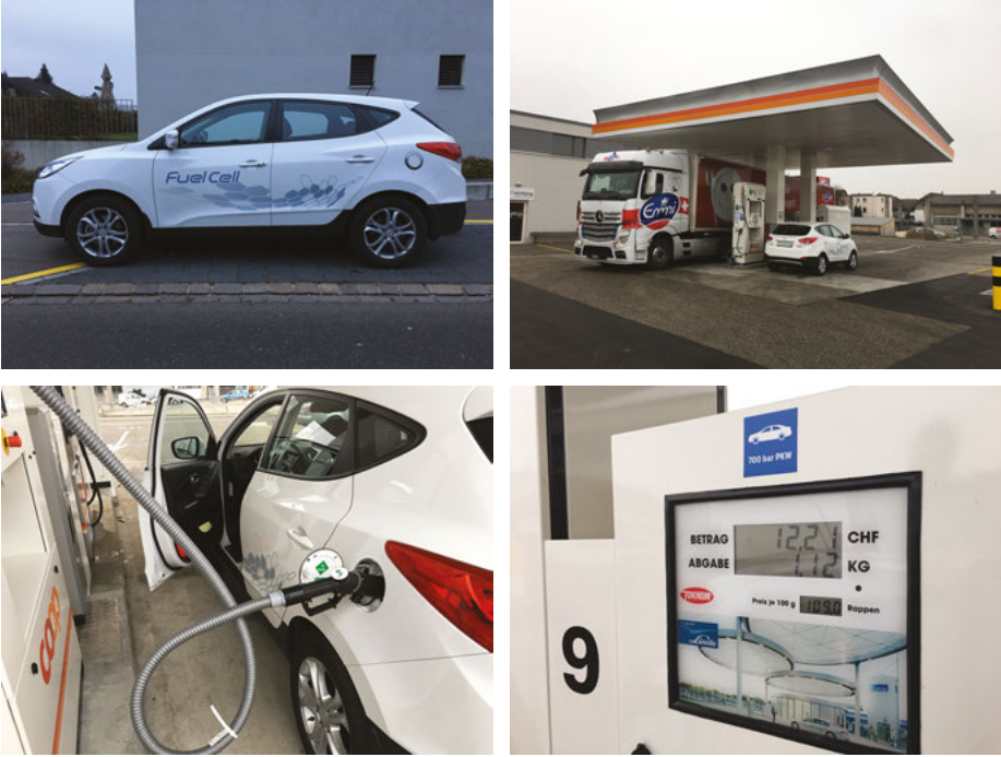
Figure 1.1: (Top left) Hyundai ix35 car in the fuel cell electric vehicle (FCEV) version with 130 hp. (Top right) The car at a hydrogen gas fueling pump station, operated by a local retail store. The hydrogen is produced by electrolysis of water with power from a hydro power plant. (Left bottom) The handle pushed into the hydrogen tank; filling takes few minutes. (Right bottom) The panel shows I have pumped 1.12 kg hydrogen for 12.21 Swiss Francs (around US $12). A full tank costs around US $50 and runs practically 400 km and nominally 596 km.
