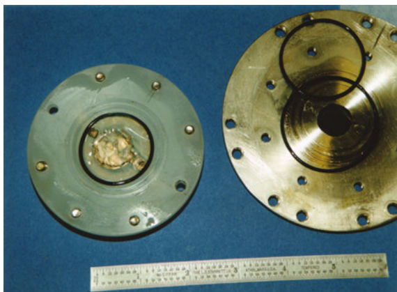
Figure 4.22: Disassembled in situ X-ray spectroelectrochemical cell with lithium metal piece on the left polypropylene plate and cathode active layer on the right stainless steel end plate Design from 1999/2000.
