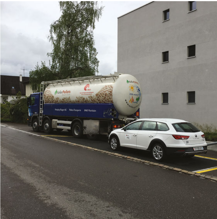
Figure 9.11: Truck delivering small pellets from compressed wood waste to a residential Minergie home near Zürich, Switzerland. The pellets are contained in the cylindrical vessel.
