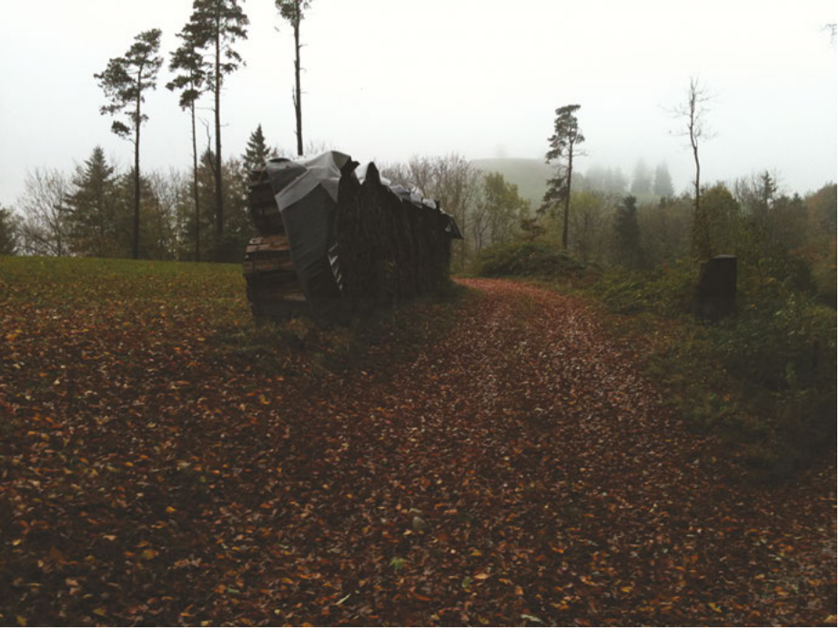
Figure 9.6: Beech wood piled up for drying in the nature at the Hulftegg Pass at the border of Kanton Zürich and Kanton Sankt Gallen, Switzerland. Plastic and metal sheets are covering the piles to protect them from excessive rain. The piles are clamped together by metal bandages for easy piling and pick up with heavy equipment.
