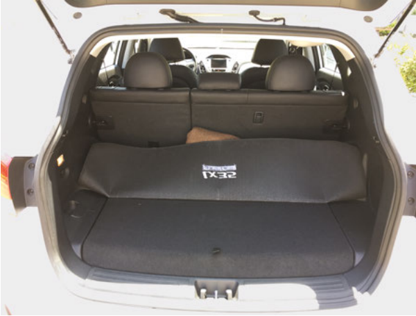
Figure 1.4: Rear space in the Hyundai ix35 Fuel Cell with the blanket put aside. Under the black panel is the hydrogen tank. Photo by Artur Braun.
