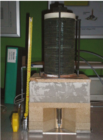
Figure 6.5: (Left) A fuel cell stack from a retired series of the Galileo system, ready for neutron tomography experiments at the Swiss Neutron Spallation Source. (Right) Schematic of an SOFC stack. The electrode assembly is a cathode from a perovskite-type metal oxide, a CGO or YSZ electrolyte layer and an anode cermet. The assemblies are connected with chromium steel plates (interconnects). Stack and Sketch provided by HEXIS AG. Photo by Artur Braun.
