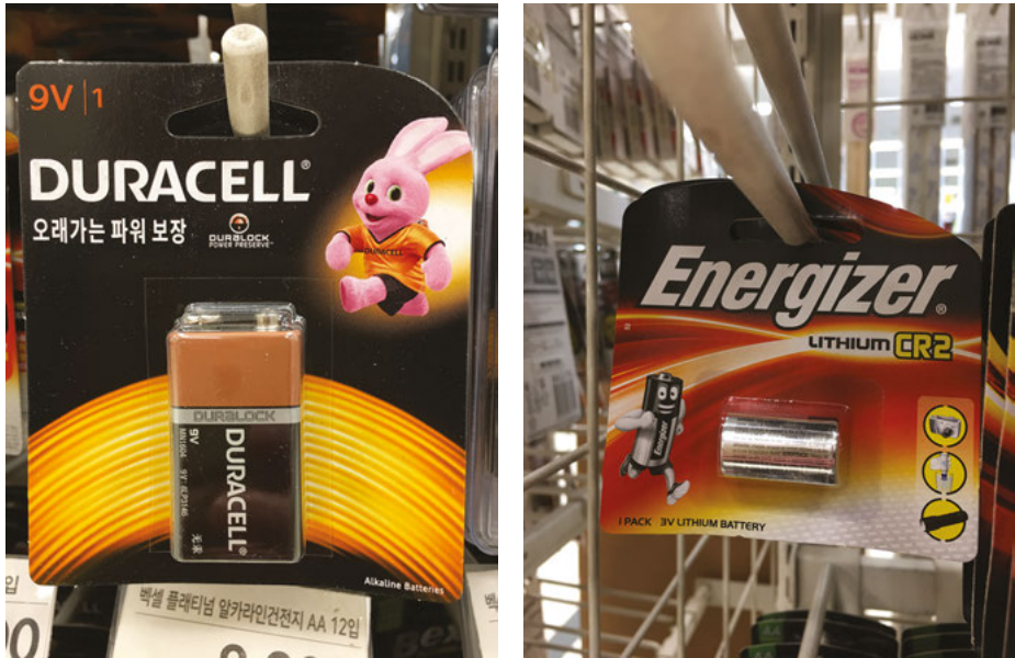
Figure 4.1: (left) DURACELL® 9V alkaline battery of type (IEC Nomenclature) MN1604, 6LP3146 (6 cells to 1.5 V each, alkaline (L) electrolyte KOH, Prismatic (P) shape with dimensions 48.5 mm × 26.2 mm × 17 mm. The cells contain Zn/MnO 2 elements. (right) Energizer® 3V battery. Notation CR means it is a lithium manganese-oxide-based battery with cylindrical C shape.
