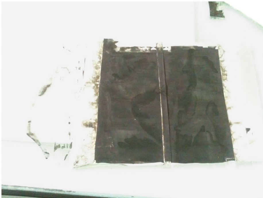
Figure 4.10: Aluminum foil coated with dried \text{LiMn}_2\text{O}_4 slurry. The rectangular shape of the dark grey slurry is obtained by putting plastic space holders and scotch tape on the aluminum foil. The space holders assist in defining a height over which you can distribute with a ruler the slurry to equal height. Produced by Dr. D.K. Bora at Empa.
