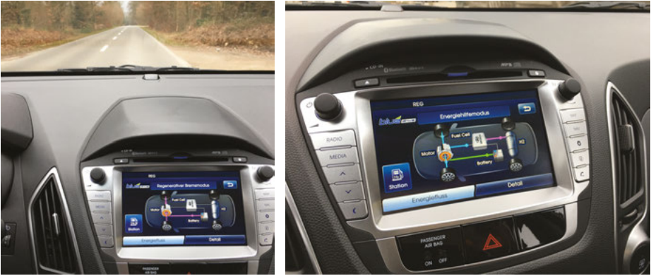
Figure 1.2: Display in the Hyundai ix35 Fuel Cell car showing the real-time energy flow between engine, battery and fuel cell.
