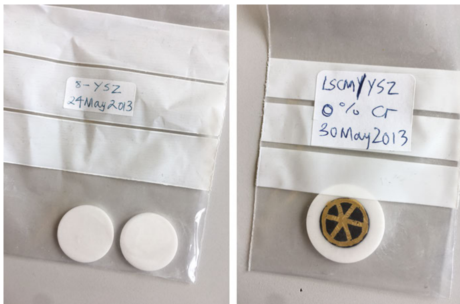
Figure 7.1: (Left) Two white pellets of 8% yttrium-stabilized zirconium oxide (8-YSZ), commercially available from some vendor. (Right) A YSZ pellet coated on the surface with a porous cathode layer from LaSrCrMn-oxide and a current collector layer from gold.
