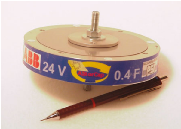
Figure 2.15: Supercapacitor prototype developed by PSI [Hahn 2001] for the Lok2000 project [Schönborn 1998]. Thirty electrodes with 150 \mu\text{m} nominal thickness and 12 cm diameter. Photo by courtesy of the Paul Scherrer Institut.
