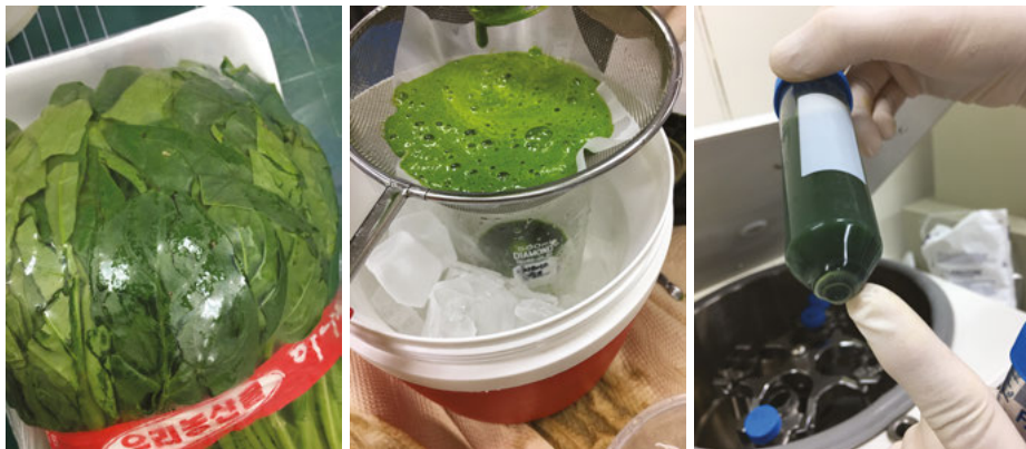
Figure 10.19: Spinach purchased from a local supermarket (Seoul, Republic of Korea) is shredded in a kitchen blender, then filtered and subject to centrifugation. Essential steps for the extraction of thylakoids from plant leaves.
