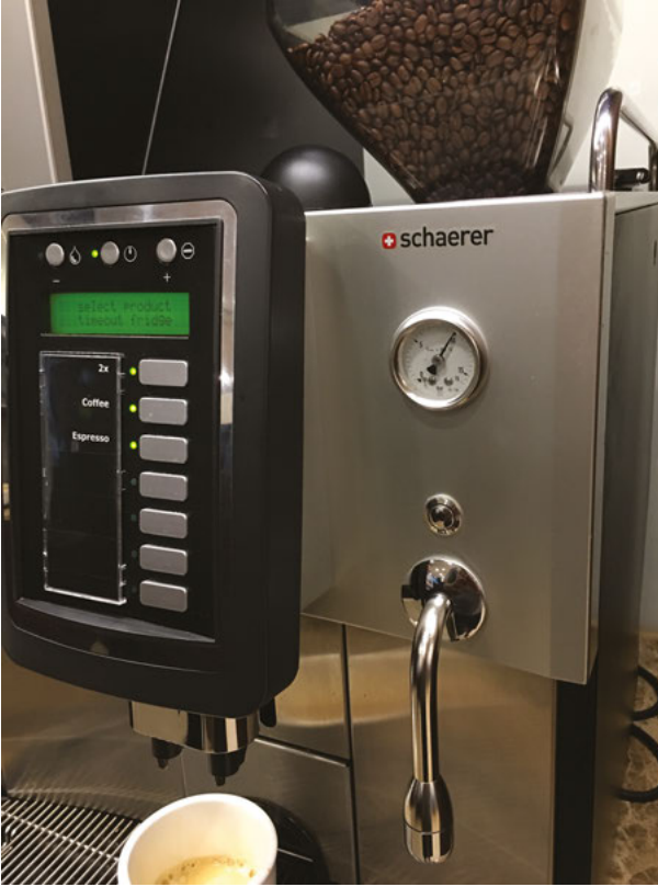
Figure 1.6: This coffee machine (Schaerer, Switzerland) used 10 bar pressure for the processing of my “espresso” coffee, as shown in the round pressure gauge on the right.
