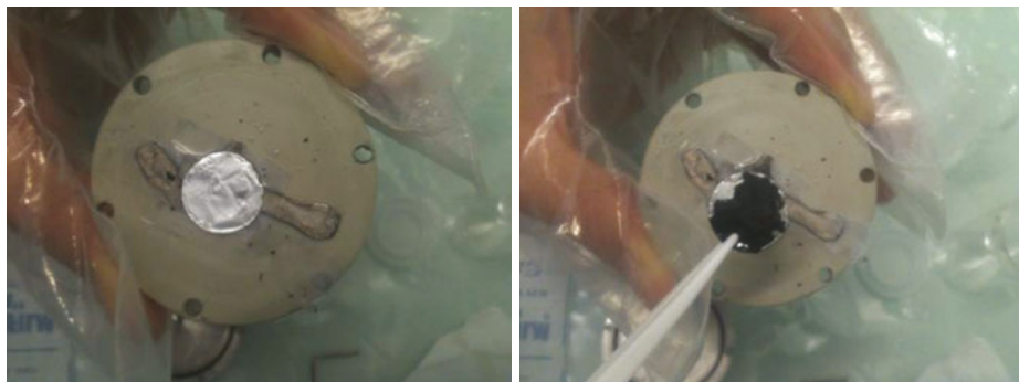
Figure 4.23: Disassembled in situ X-ray spectroelectrochemical cell (design from 2012) inside a glove bag. The cell was used for the study reported in [Braun 2015].
