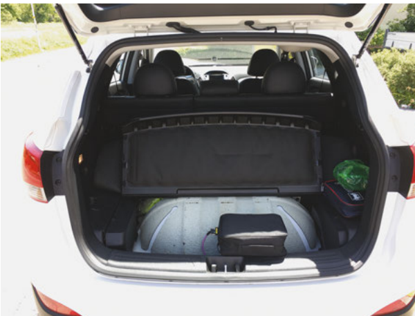
Figure 1.5: Rear space in the Hyundai ix35 Fuel Cell with the back cover opened. The white roundish container is the hydrogen storage tank that can sustain the 700 bar pressure. It can contain around 5.64 kg H 2 at this pressure. Photo by Artur Braun.
