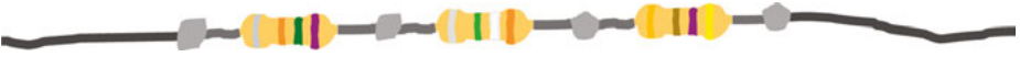
Figure 5.3: Illustration of three resistors R_1 , R_2 and R_3 soldered together in series between two wires. The colors on the resistors specify their resistivity including the tolerance (error). The color code is shown in the Appendix and can be used to find out the resistance.
