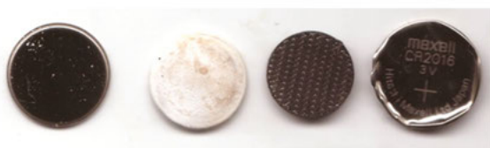
Figure 4.9: Disassembled primary lithium battery from Maxell. Top row shows stainless steel current collector and end plate from inside with corroded lithium metal. The white disk is the separator. The black smaller disc is the active electrode material. The black metal disk shows the other stainless steel end plate from inside, with traces from the black active material.
