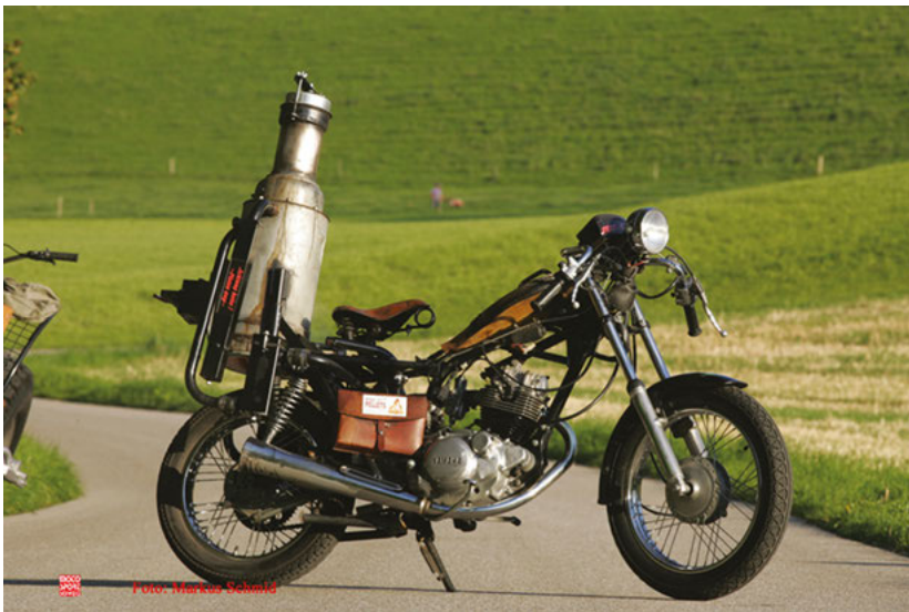
Figure 9.14: Yamaha motor bike equipped with a wood gas reactor.
