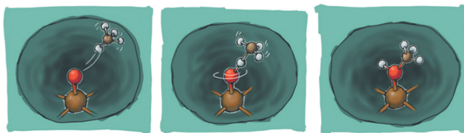
Scheme 1 Proposed reaction mechanism of methane hydroxylation by [\text{FeO}]^{2+} -exchanged zeolites via a homolytic H-atom abstraction leading to the formation of a methyl radical and a subsequent methanol molecule. Adapted with permission from ref. 90. Copyright 2016 American Chemical Society.
