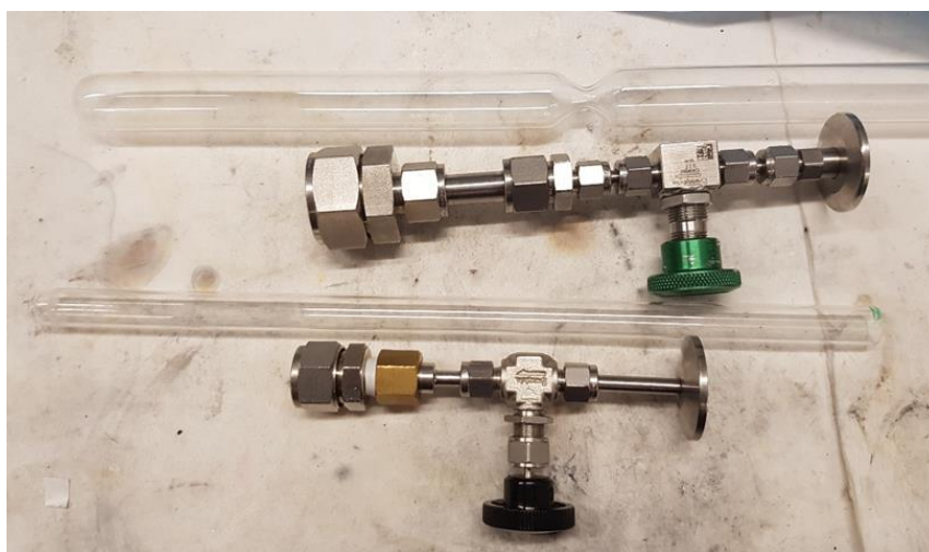
Figure 2.1. Picture showing the Swagelok setup and quartz ampoule for both the larger and smaller tubes
