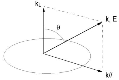
The knowledge of E and then  $|\mathbf{k}_i|$  allows one to get the band structure diagram  $E \to \mathbf{k}$  (wavevector).
