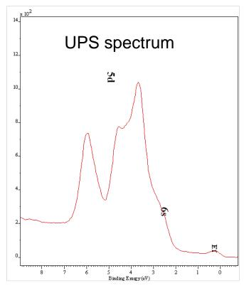
In general, *the energy dependence* of the photoionization cross-section can be exploited to see that some features are enhanced in UPS and others are suppressed. The situation is reversed in XPS
