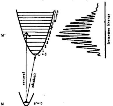
Potential energy curves with vibrational levels showing the origin of the vibrational structure of the photoelectron band. The vertical and adiabatic ionization energies are indicated
