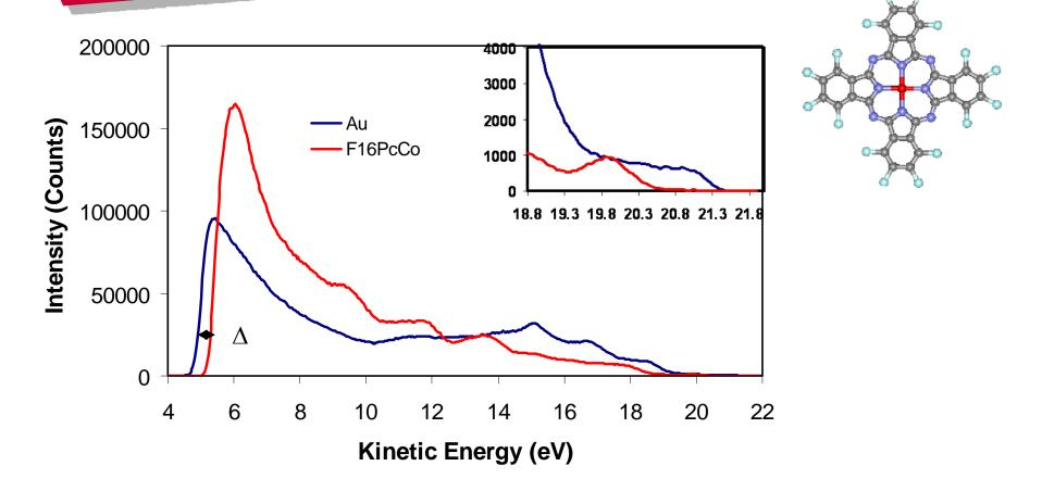
A vacuum shift  $\Delta = 0.5$  eV was measured at the lower KE side of the UPS spectrum obtained for the compound.
