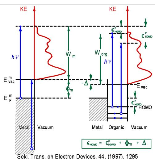
Energy relationship cartoon, left for Au, right for an organic layer deposited on the metal substrate.
