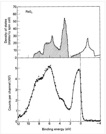
(*p-derived* features are generally suppressed in XPS and strong *d-hybridized* features enhanced).
