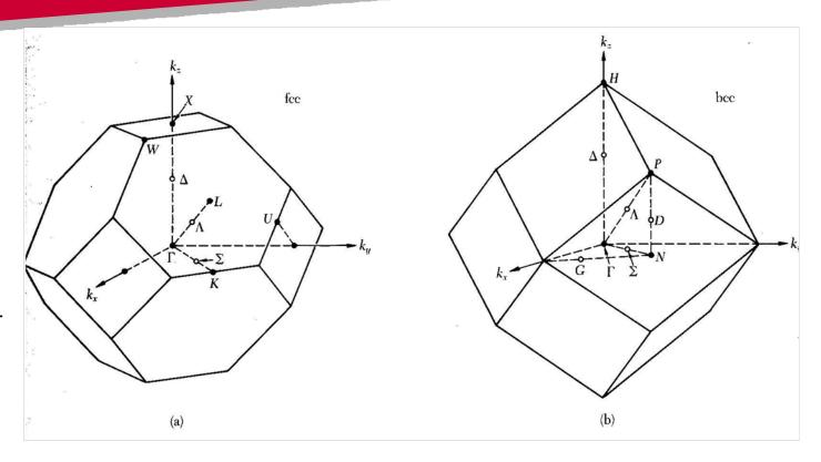
In (a) the boundary point at  $2\pi/a$  (100) is X; the boundary point at  $2\pi/a$  (1/2,1/2,1/2) is L, the line  $\Delta$  runs between  $\Gamma$  and X.
