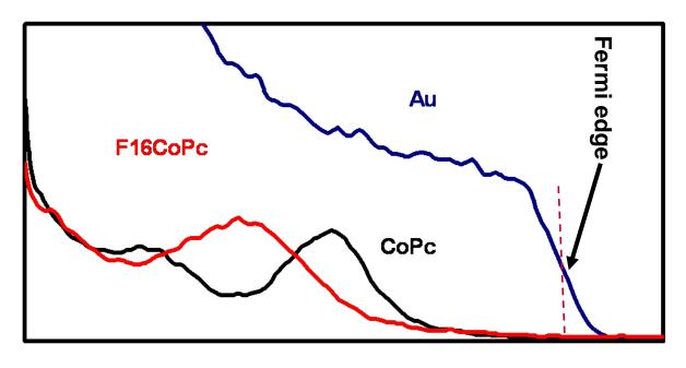
UPS data shows the first ionization energies for CoPc and  $F_{16}$ CoPc (HOMO) adsorbed on Au surface. A difference of 0.5 eV was measured between CoPc and F16CoPc compounds. This is due to the high electro-negativity of fluorine (highest withdrawing electron power than of H) therefore the electrons are tightly bound  $\rightarrow$  need more energy (higher KE).
