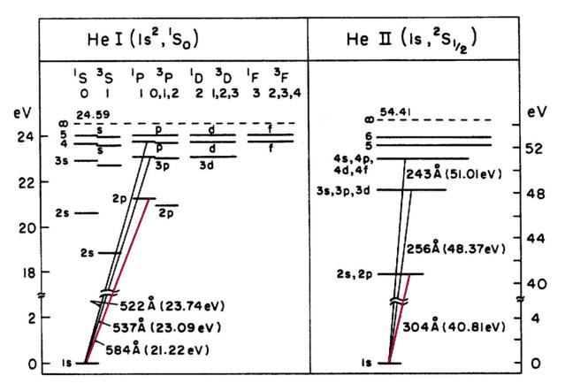
Grotian diagram for He I and He II showing the strongest resonance lines (584 Å, 98% of the emission intensity, the other lines present in a He discharge are 537 Å, 522 Å and 304 Å which can have intensity of the order of 2 % of the 584 Å line.
