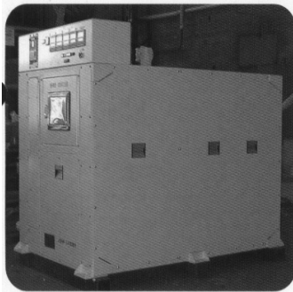
Fig. 40: JSW large (75 Nm 3 H 2 ) Metal-Hydride tank with water cooling
