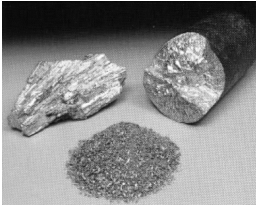
Fig. 7: Metal-hydride based intermetallic alloys are melted into ingots, which are then crushed or decrepitated with hydrogen into powders
