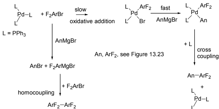
Figure 13.24. Slow addition of Grignard suppresses homo-coupling
