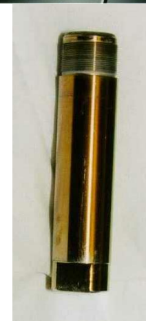
sample holder L = 70 mm Ø = 15 mm
