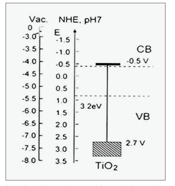
Fig.1. The positions of bottom of the conduction band and top of the valence band for  $\text{TiO}_2$  semiconductor. The potential values are given both in electrochemical scale and absolute scale on the left. On the right the water decomposition potentials to evolve hydrogen and oxygen are given at a pH value of 7.
