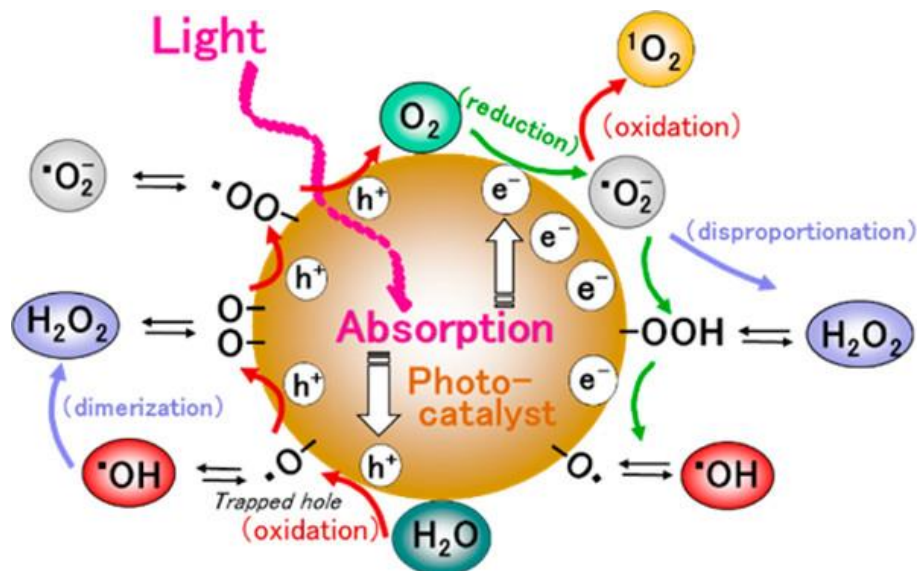
Fig. (10). Pictorial representation of generation of Reactive Oxygen Species on photo-catalytic semiconductor surfaces.
