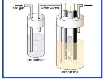
not perturbing the solution in the cell. Another option is to feed electrode cables into an inert atmosphere glovebox and run electrochemical experiments using previously deoxygenated solvents.
