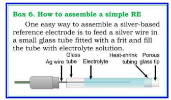
presumably takes advantage of the natural oxide layer on the silver wire, using the resulting ill-defined  $Ag_2O/Ag$  couple. This method eliminates the possibility of silver salts leaks but requires the presence of an internal standard.
