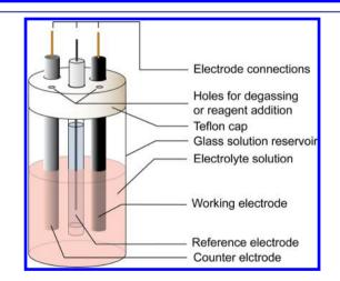
Figure 4. Schematic representation of an electrochemical cell for CV experiments.
