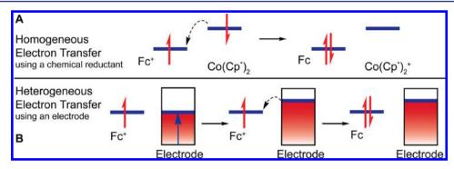
Figure 1. (A) Homogeneous and (B) heterogeneous reduction of  $Fc^+$  to Fc. The energy of the electrons in the electrode is controlled by the potentiostat; their energy can be increased until electron transfer becomes favorable.<sup>4</sup>
